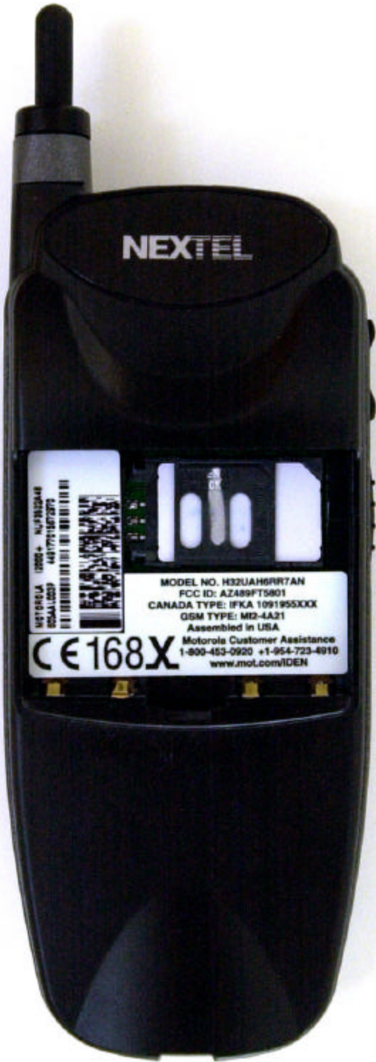
Photograph 3-3: Rear view of the radio, showing FCC label
