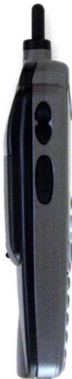
Photograph 3-2: Side view of the radio with NTN8615 battery (additional batteries listed in Exhibit 12.2.1)
