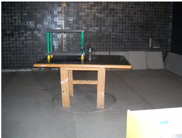
Photograph 7.1.1 Setup for spurious emission field strength measurements
