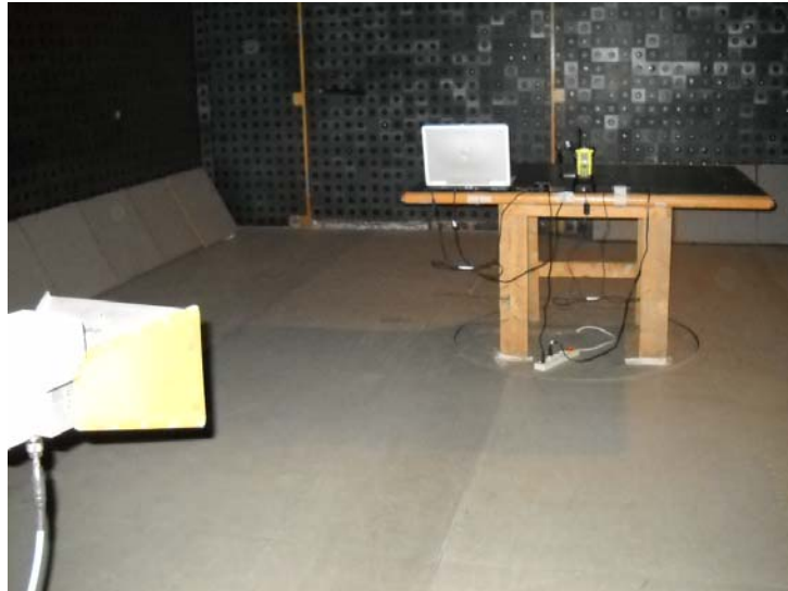
Photograph 7.7.3 Setup for spurious emission field strength measurements above 1000 MHz
