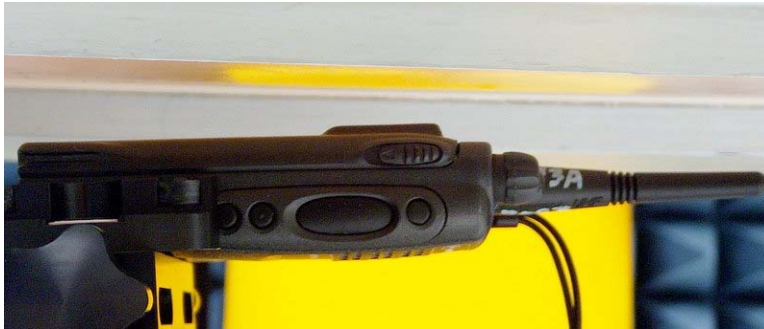
Figure 3: Body Assessment DUT back w/ antenna separated 2.5cm from the phantom, Worst case audio acc. Model RMN4029A w/ RLN4922A attached.
