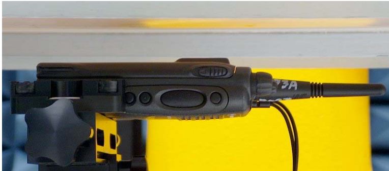
Figure 5: Body Assessment DUT w/ front housing separated 2.5cm from the phantom, Worst case audio acc. Model RMN4029A w/ RLN4922A attached.
