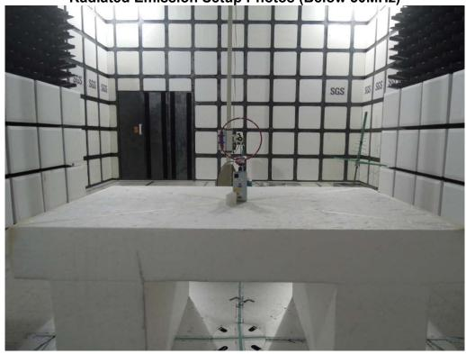
Radiated Emission Setup Photos (30MHz~1GHz)
