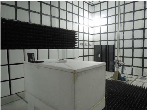
Radiated Emission Set up Photos (Front View)
