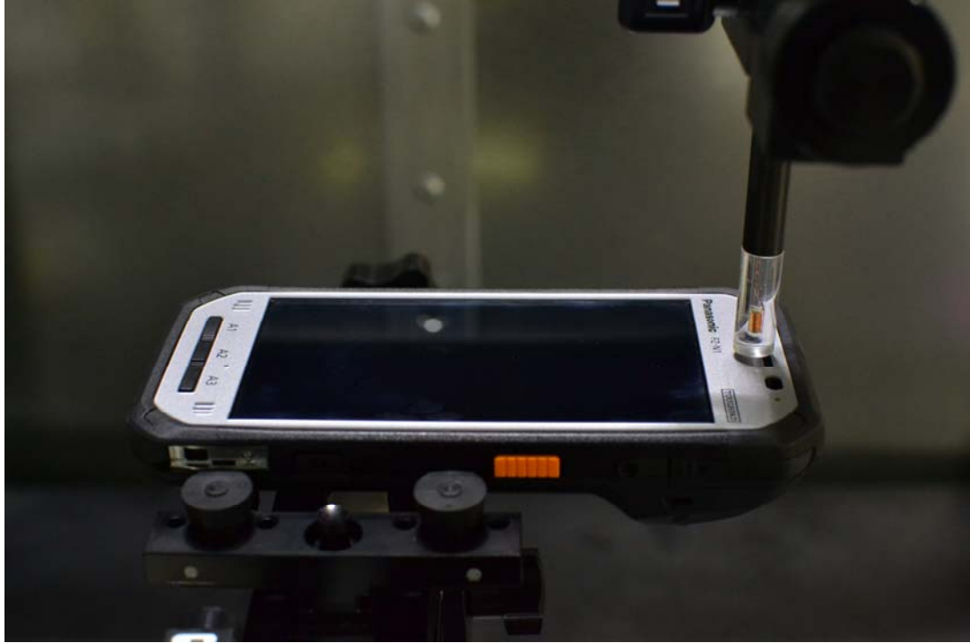
Figure 14-1 Test Setup for Wireless Device (Standard Battery)
