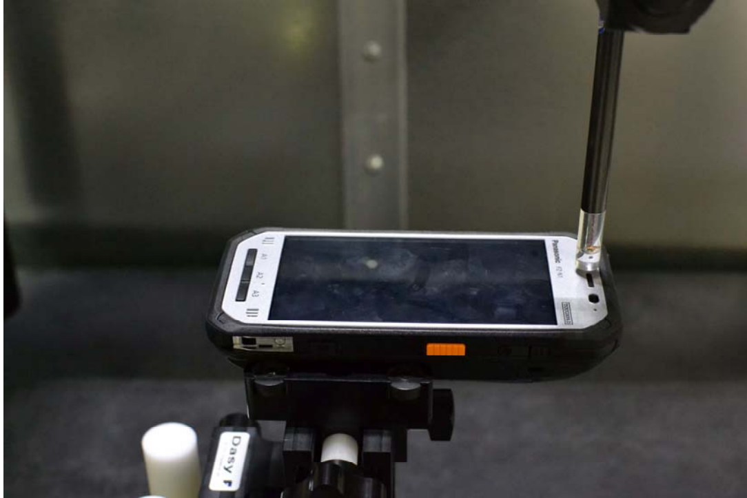
Figure 14-3 Test Setup for Wireless Device (L-Battery)
