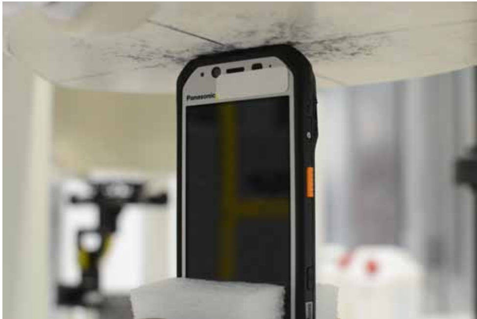
SAR Test Setup Photo 20 – Top Edge at 0.0 cm with Standard Battery
