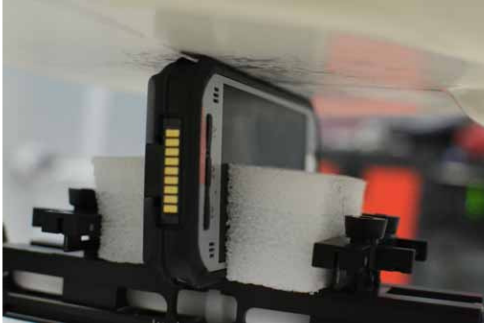
SAR Test Setup Photo 27 – Left Edge at 0.0 cm with L-Battery
