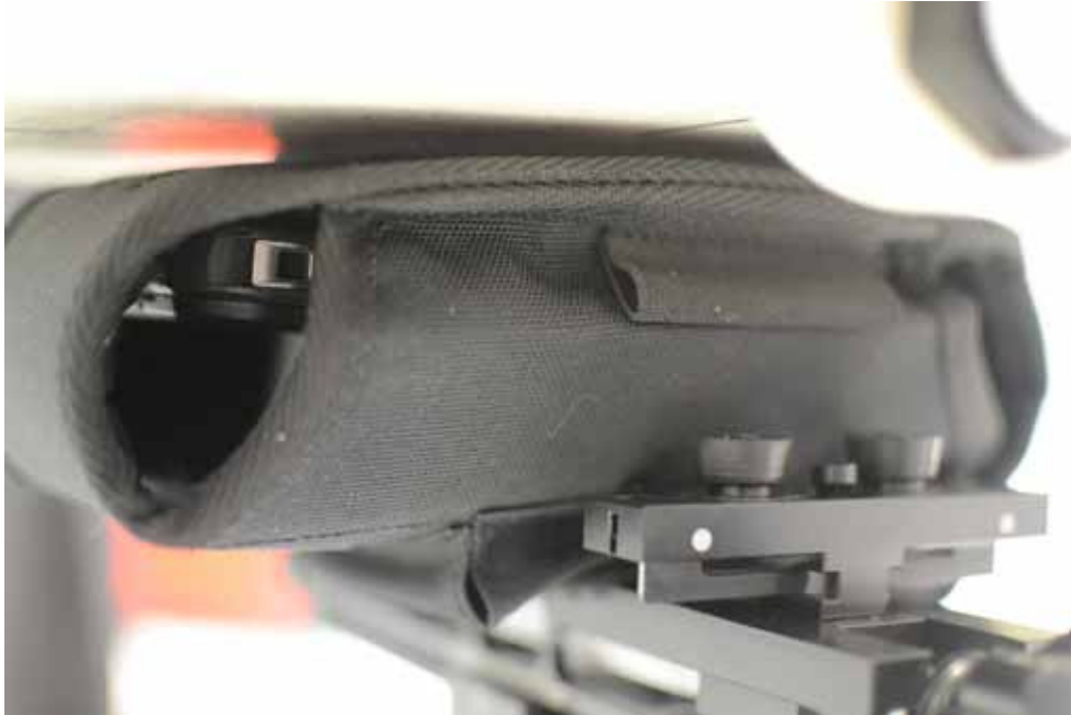
SAR Test Setup Photo 17 – Front Side at 0.0 cm with Standard Battery and Body Holster Accessory
