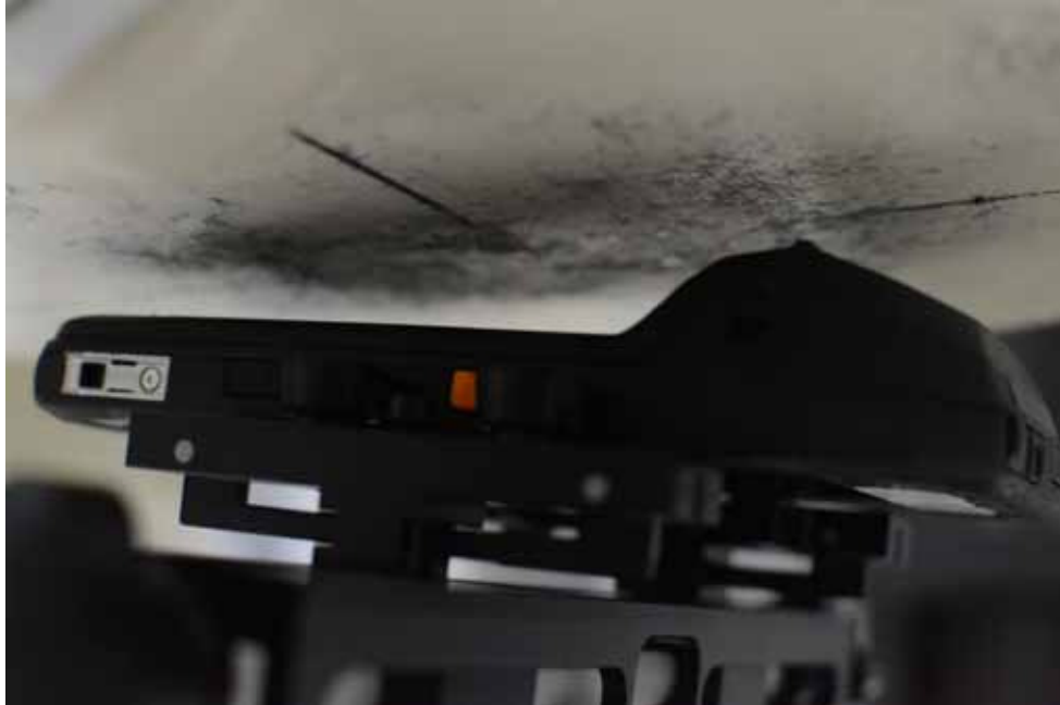
SAR Test Setup Photo 7 – Back Side at 1.0 cm with Standard Battery
