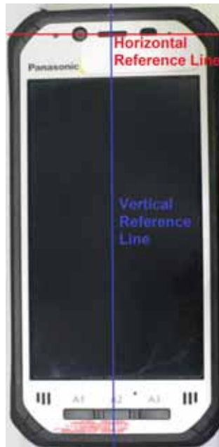
SAR Test Setup Photo 28 – Horizontal and Vertical Reference Lines
