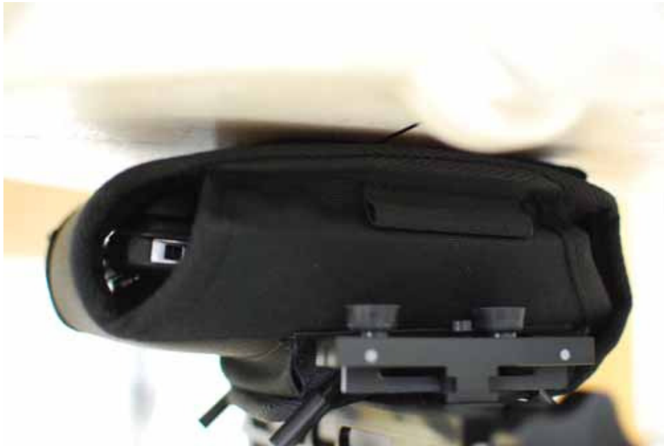
SAR Test Setup Photo 12 – Back Side at 0.0 with L-Battery and Body Holster Accessory
