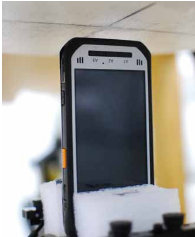
SAR Test Setup Photo 22 – Bottom Edge at 1.0 cm with Standard Battery
