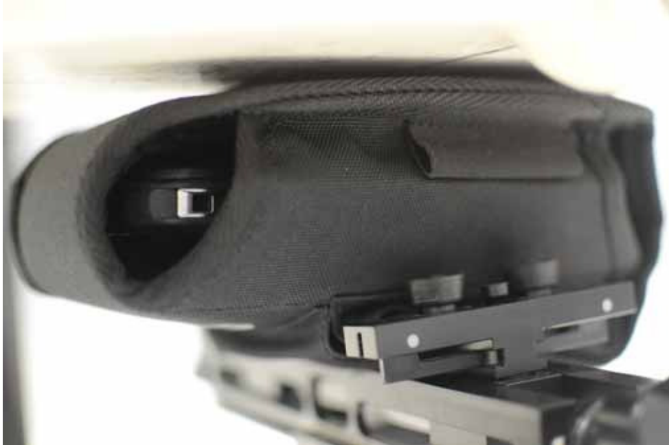
SAR Test Setup Photo 11 – Back Side at 0.0 with Standard Battery and Body Holster Accessory
