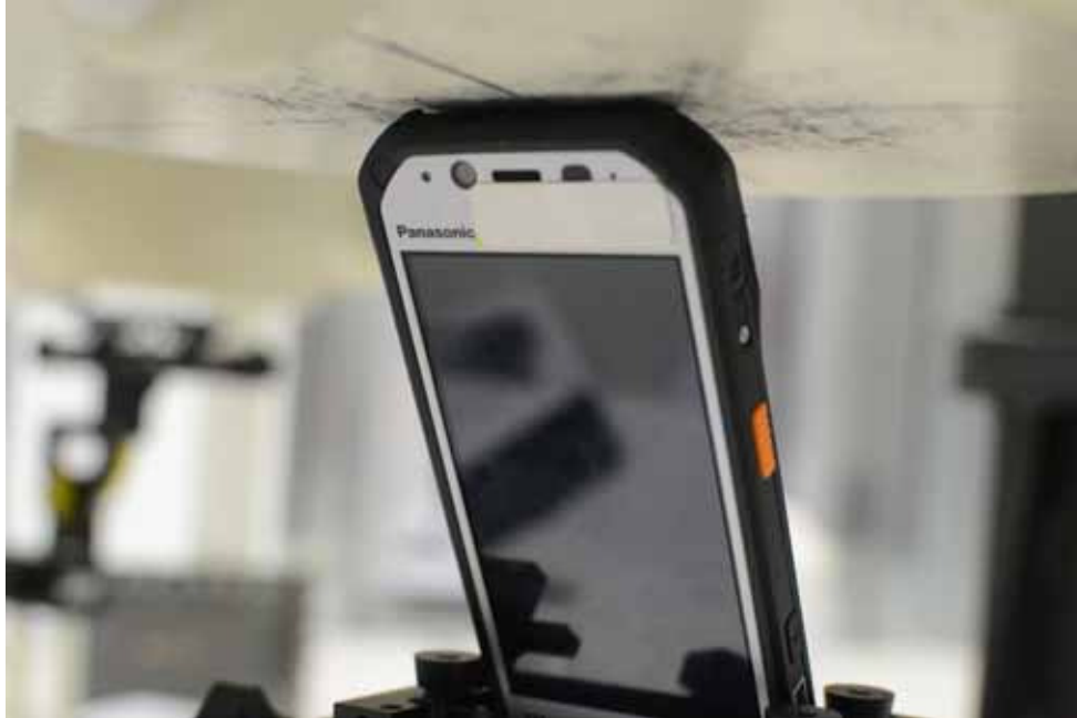
SAR Test Setup Photo 21 – Top Edge (Tilt) at 0.0 cm with Standard Battery
