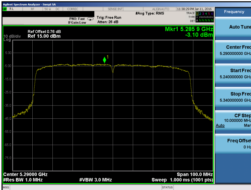
Plot 7-56. Power Spectral Density Plot (80MHz BW 802.11ac (UNII Band 2A) – Ch. 58)
