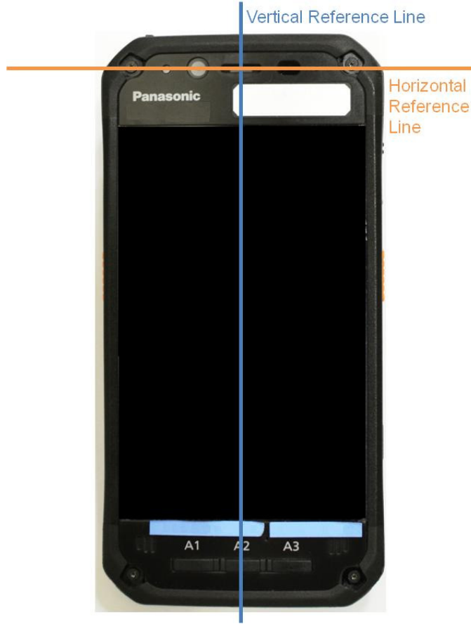
SAR Test Setup Photo 15: Horizontal and Vertical Reference Lines
