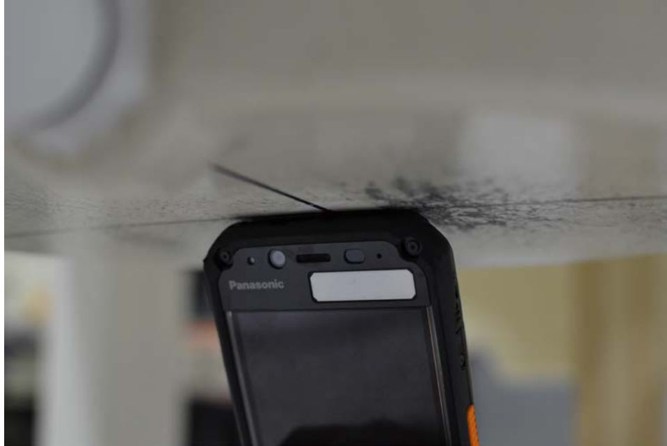
SAR Test Setup Photo 13: Top Edge (Tilt) at 0.0 cm
