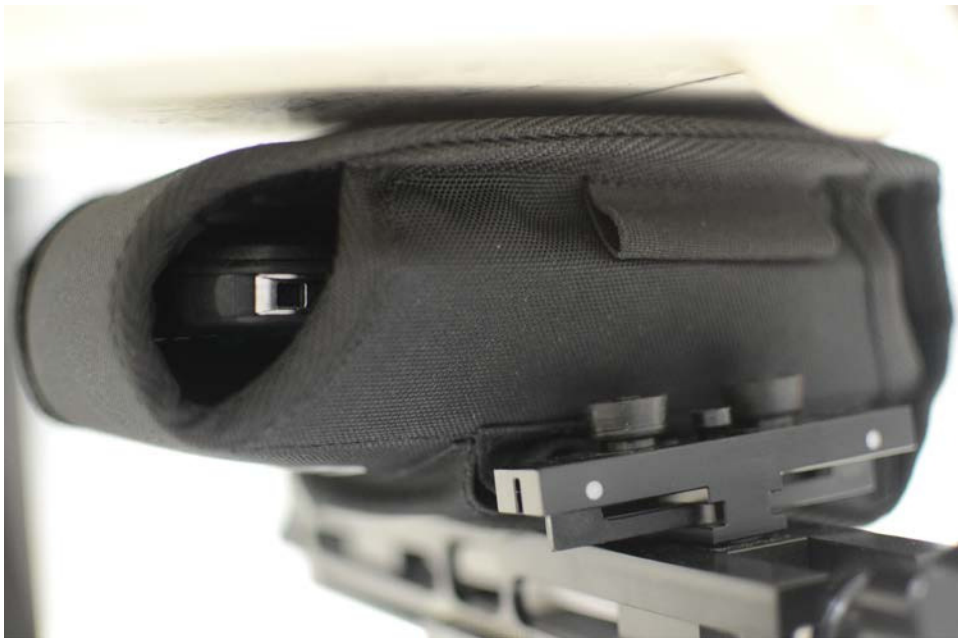
SAR Test Setup Photo 8: Back Side at 0.0 cm with Body Holster Accessory
