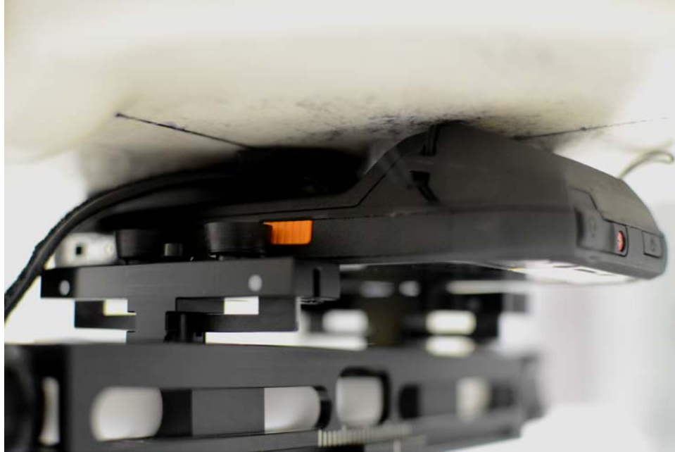
SAR Test Setup Photo 9: Back Side at 0.0 cm with Hand Strap Accessory
