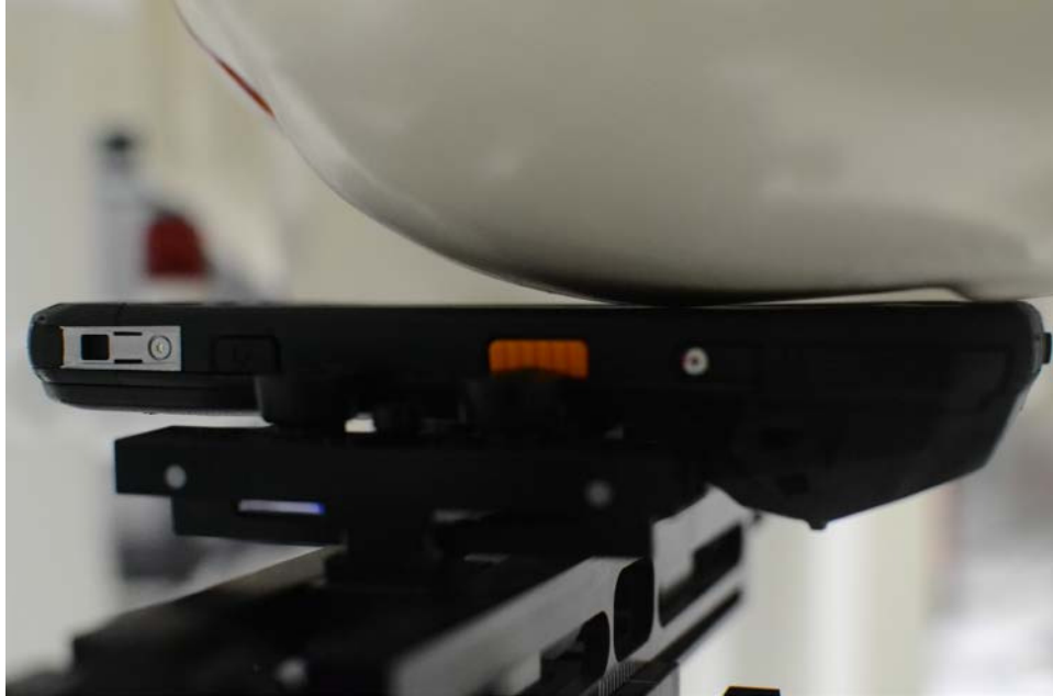
SAR Test Setup Photo 3: Left Cheek
