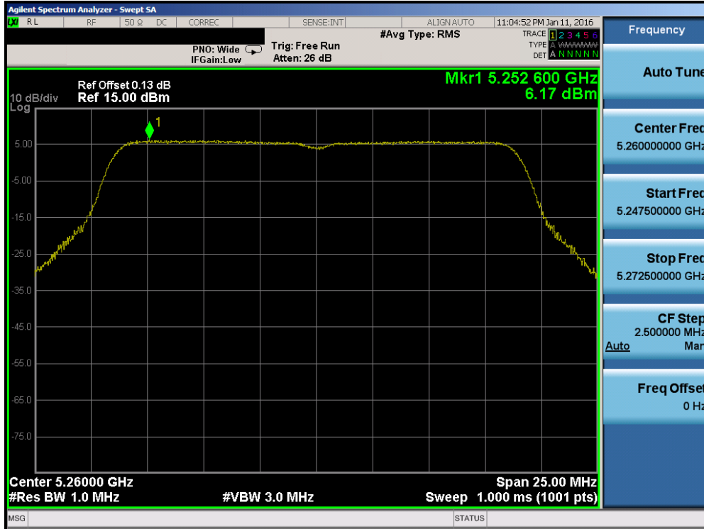
Plot 7-51. Power Spectral Density Plot (20MHz BW 802.11n (UNII Band 2A) – Ch. 52)
