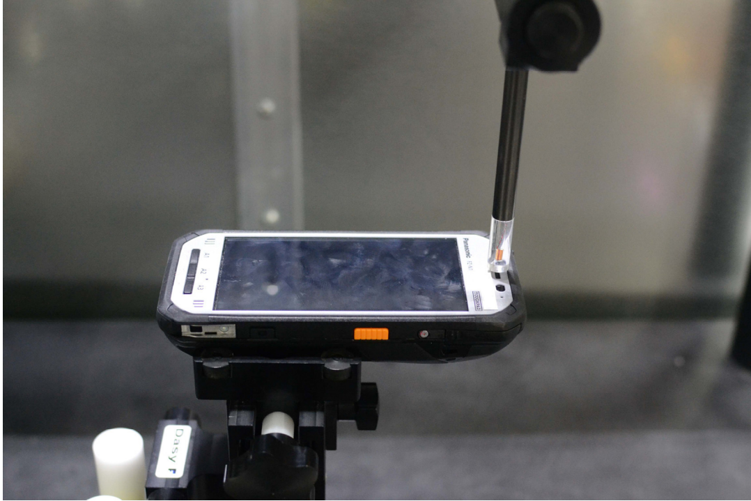
Figure 14-3 Test Setup for Wireless Device (L-Battery)
