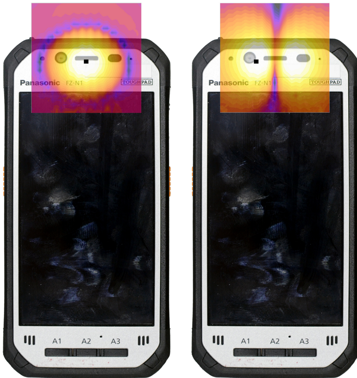
Figure 14-5 T-Coil Scan Overlay Magnetic Field Distributions
