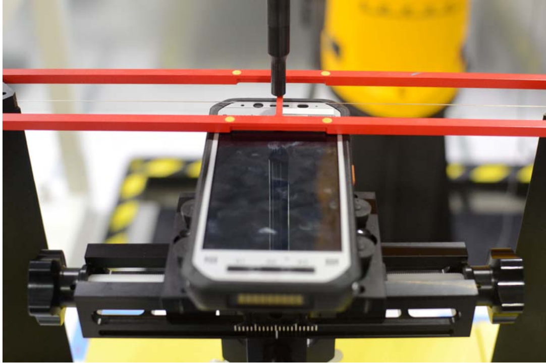
Figure 18-3 Ear Reference Point HAC Phantom Alignment (L-Battery Accessory)
