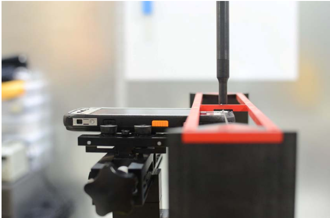
Figure 18-2 HAC Phantom Plane Alignment (Standard Battery)
