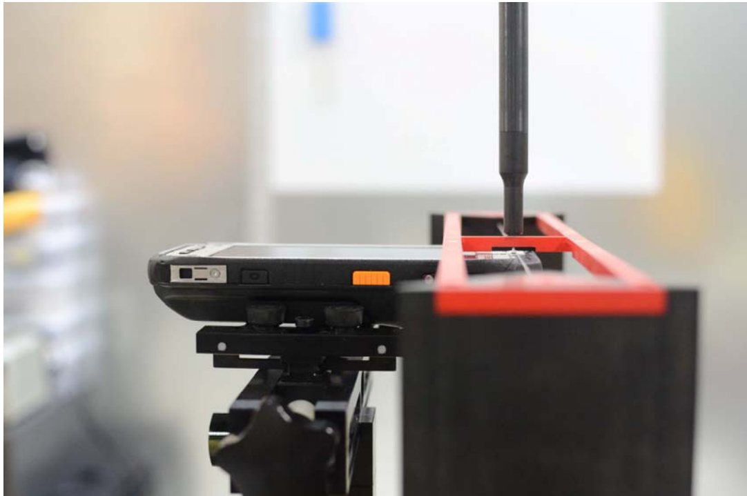
Figure 18-4 HAC Phantom Plane Alignment (L-Battery Accessory)
