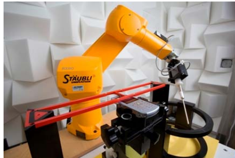
Figure 5-3 SPEAG Robotic System
