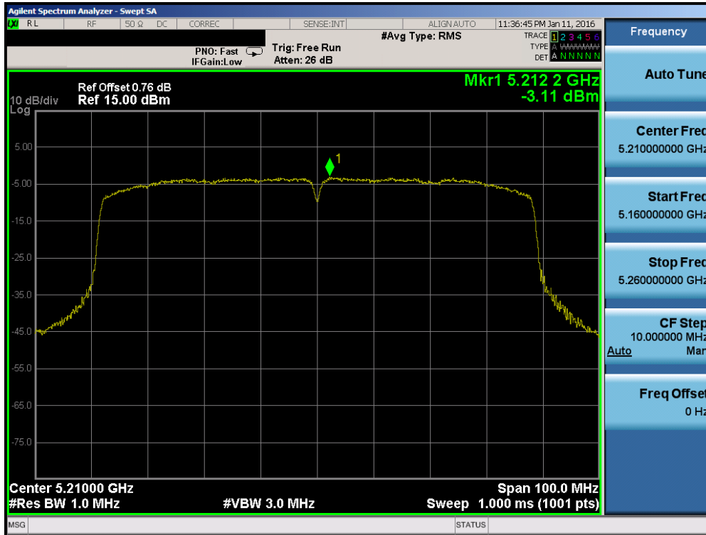
Plot 7-47. Power Spectral Density Plot (80MHz BW 802.11ac (UNII Band 1) – Ch. 42)
