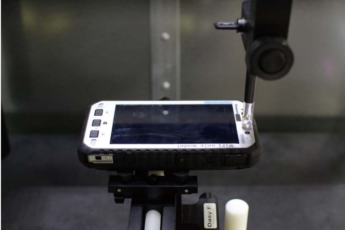
Figure 14-1 Test Setup for Wireless Device
