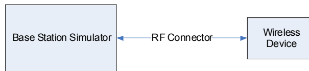
Figure 9-3 Power Measurement Setup
