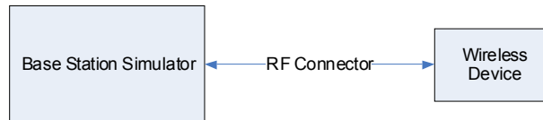
Figure 9-2 Power Measurement Setup
