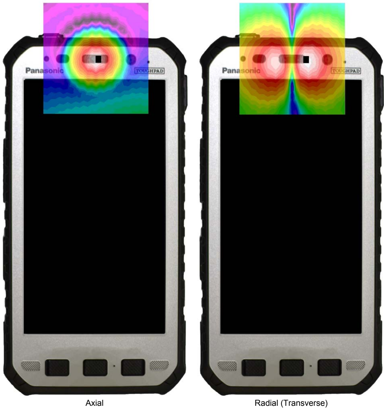
Figure 13-3 T-Coil Scan Overlay Magnetic Field Distributions
