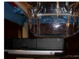
Figure 14.1 Body SAR Lap Position Test Setup
