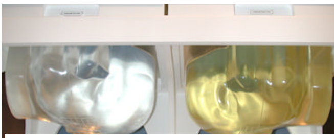
Figure 7.1 Left and Right SAM Phantom shells
