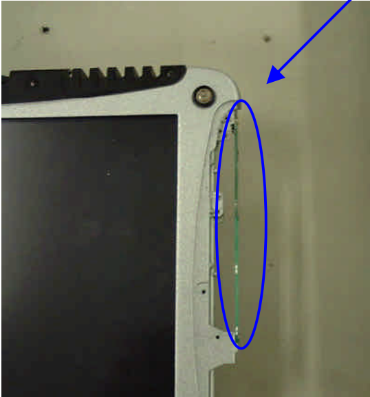
Antenna cover open view
