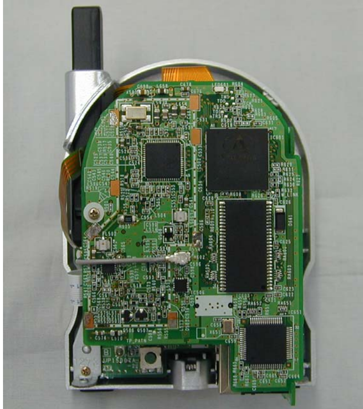
Module with Antenna Cable
