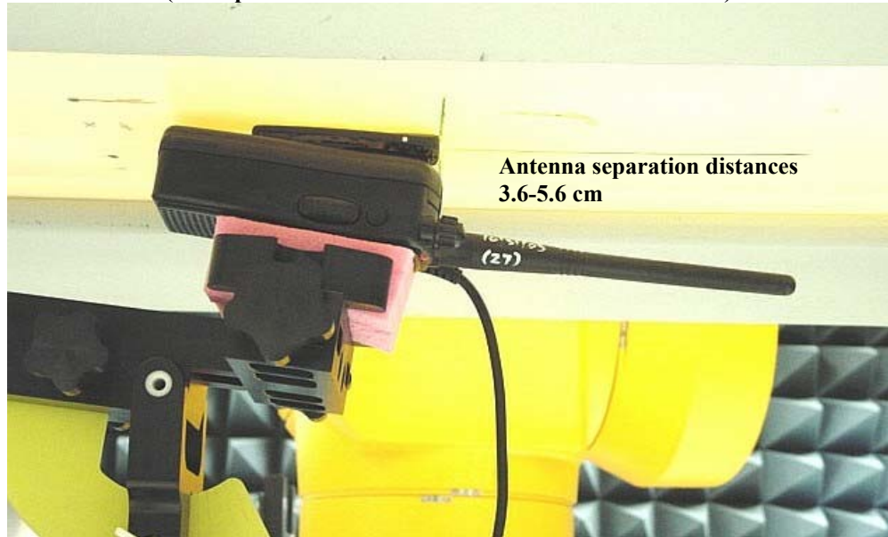
Figure 2. Assessment @ the body; DUT w/ belt clip model HLN9844A against the flat phantom with antenna model PMAD4015A and attached audio accessory model HMN9030A (Same position used to assess the other offered antenna)
