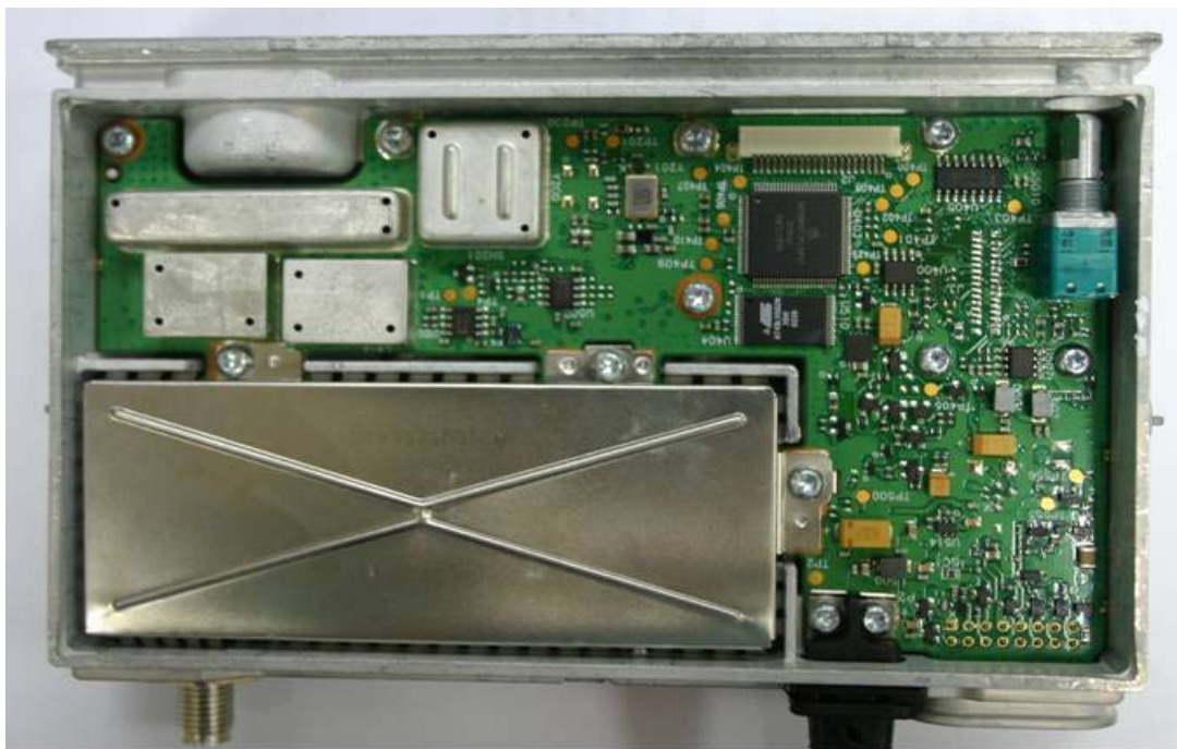
Figure 9-6: Top View of PCB placed in chassis with shield covering transmitter section.
