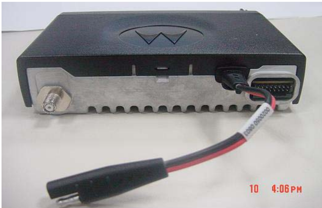
Figure 3-5: Rear view showing antenna connector, DC cable, and accessory connector
