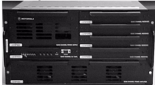
Figure:1-2 QUAD Channel Base Radio (Typical)
