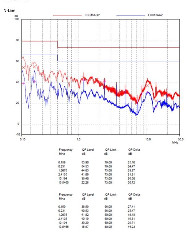
Remark: 1. Correct Factor = LISN Factor + Cable Loss, the value was added to Original Receiver Reading by the software automatically.
