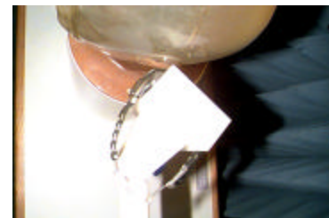
Fig. 14 Head SAR Test Setup
