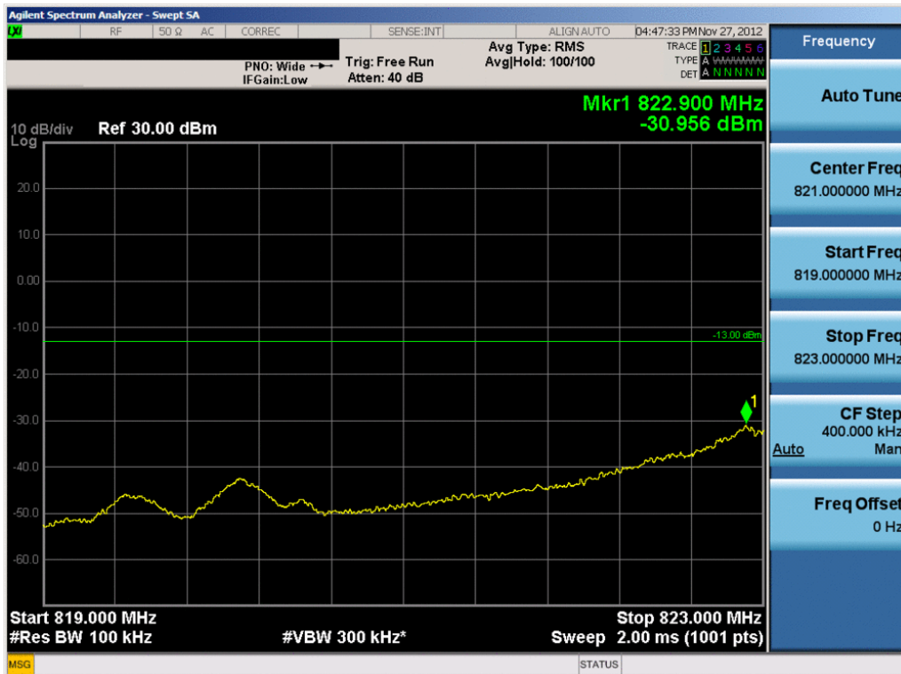
Plot 7-26. 4MHz Span Plot (Cellular CDMA Mode – Ch. 1013)
