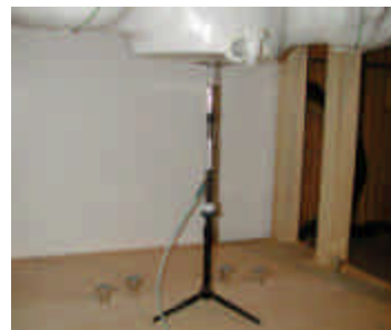
Figure 12.1 Dipole Validation Test Setup
