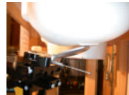
Figure 14.8 Left Head SAR Test Setup -- Ear / Tilt Position --
