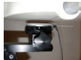
Figure 14.13 Body SAR Test Setup -- w/ Belt-clip --
