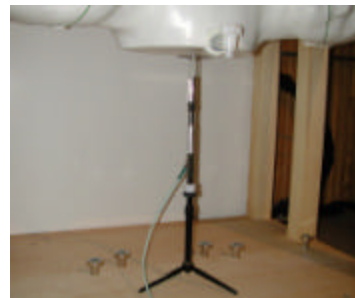
Figure 12.1 Dipole Validation Test Setup
