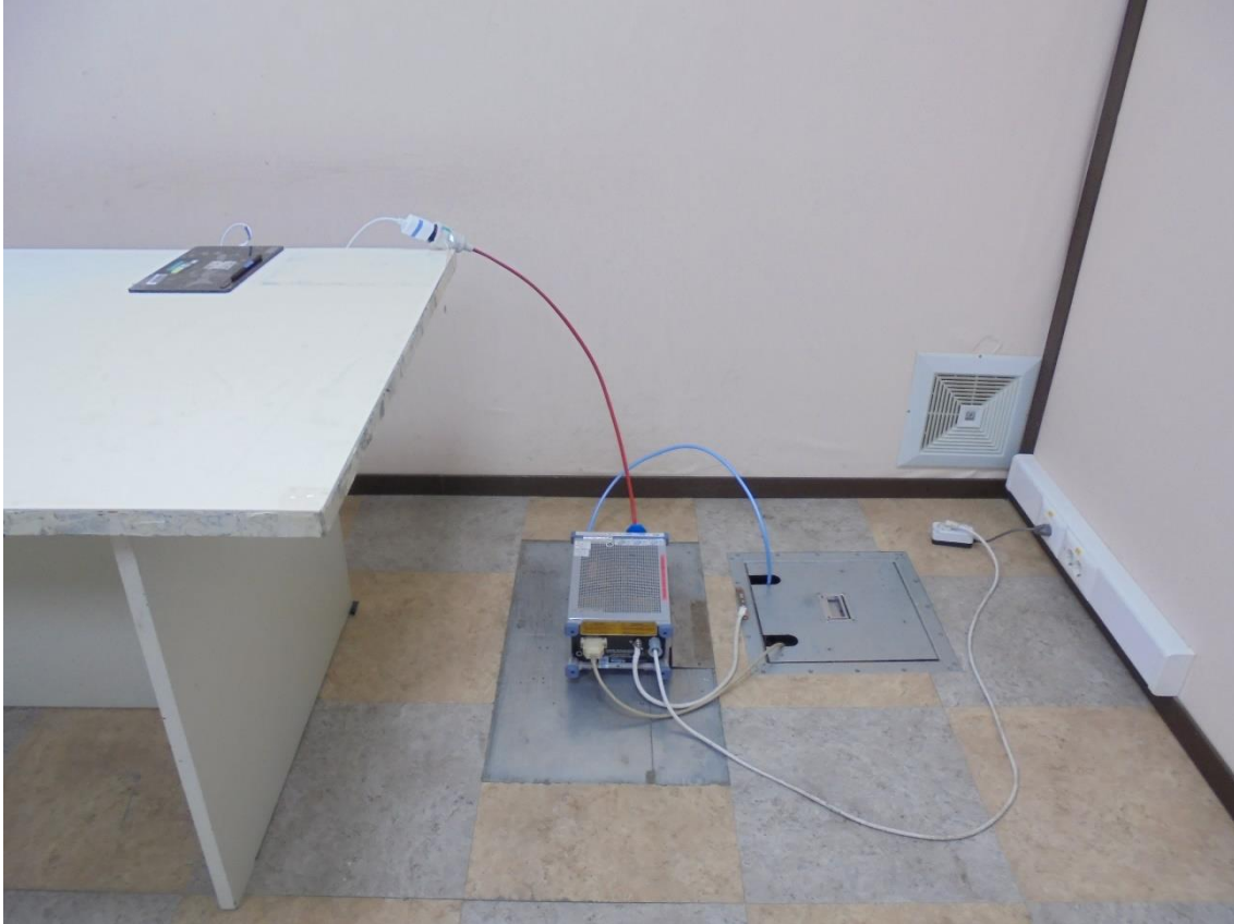
AC Power Line Conducted Test WPT (S-Pen) Setup Photo
