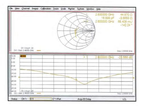
**Calibration for Impedance and Return-loss**
