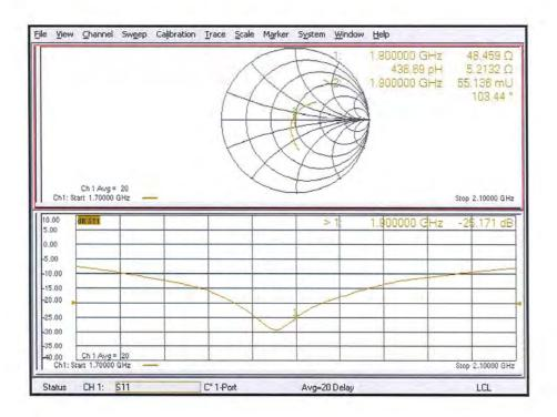
**Calibration for Impedance and Return-loss**
