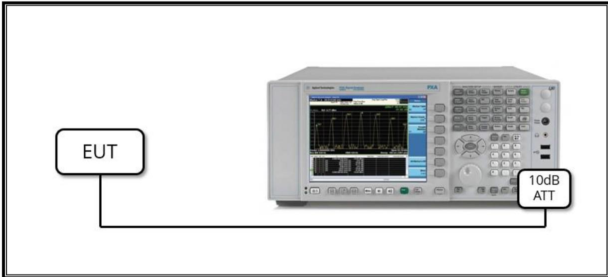
**SETUP DIAGRAM FOR TESTS (RADIATED TEST SETUP)**
