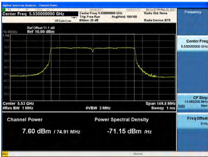
802.11ac_VHT80 UNII 2C BAND Average Power (5530 MHz) CH 106 MCS3
