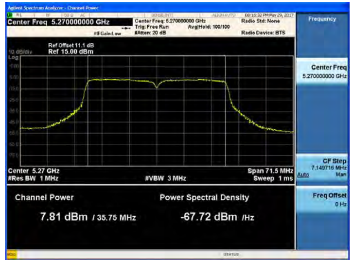
802.11ac_VHT40 UNII 3 BAND Average Power (5755 MHz ~5795 MHz) CH 151 MCS5
