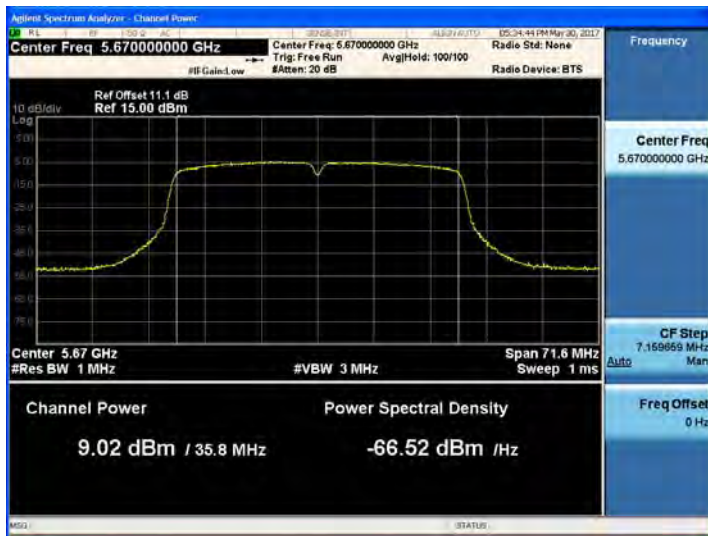
802.11n_HT40 UNII 2C BAND Average Power (5510 MHz ~5670 MHz) CH 134 MCS1
