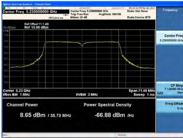
802.11n_HT40 UNII 2C BAND Average Power (5510 MHz ~5670 MHz) CH 134 MCS1
