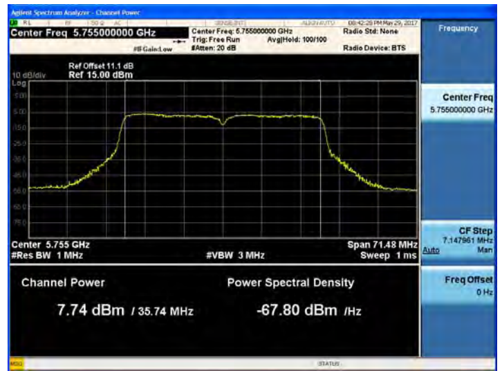
802.11ac_VHT40 UNII 3 BAND Average Power (5755 MHz ~5795 MHz) CH 151 MCS5
