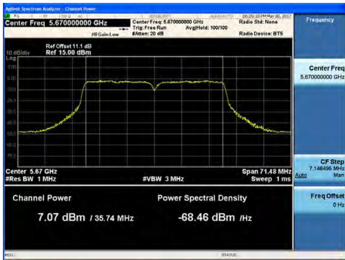
802.11ac_VHT40 UNII 2C BAND Average Power (5510 MHz ~5670 MHz) CH 134 MCS8
