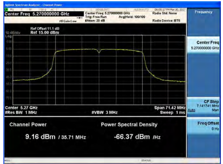
802.11ac_VHT40 UNII 3 BAND Average Power (5755 MHz ~5795 MHz) CH 159 MCS1
