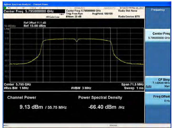
802.11ac_VHT40 UNII 3 BAND Average Power (5755 MHz ~5795 MHz) CH 159 MCS1
