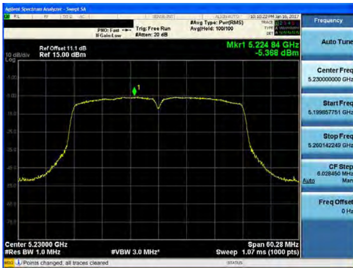
802.11ac_VHT40 UNII 2C BAND PSD CH 110
