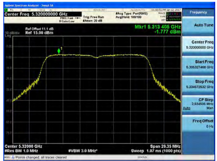
802.11ac_VHT20 UNII 3 BAND PSD CH 165
