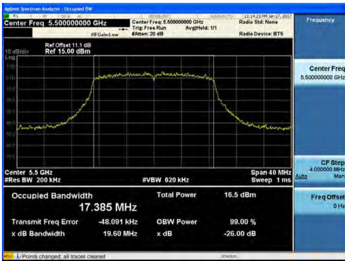
802.11n_HT20 UNII 2C BAND 26dB Bandwidth(CH 100)
