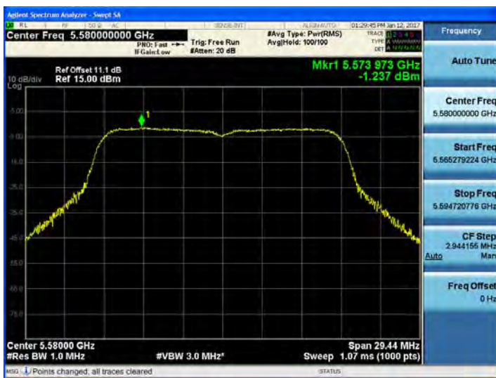
802.11ac_VHT20 UNII 2C BAND PSD CH 116
