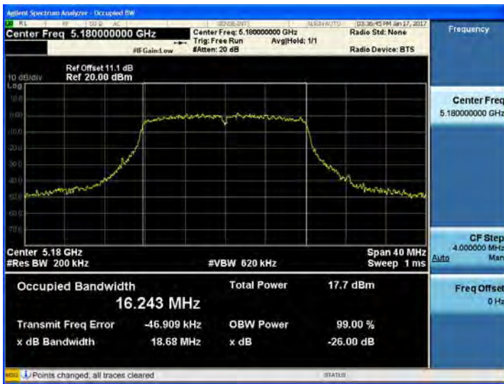
802.11a UNII 2C BAND 26dB Bandwidth (CH 100)
