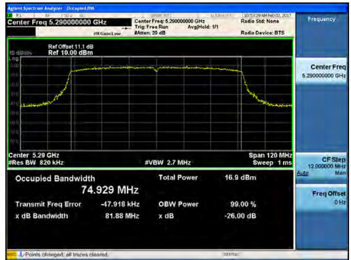
802.11ac_VHT80 UNII 3 BAND 26dB Bandwidth(CH 155)
