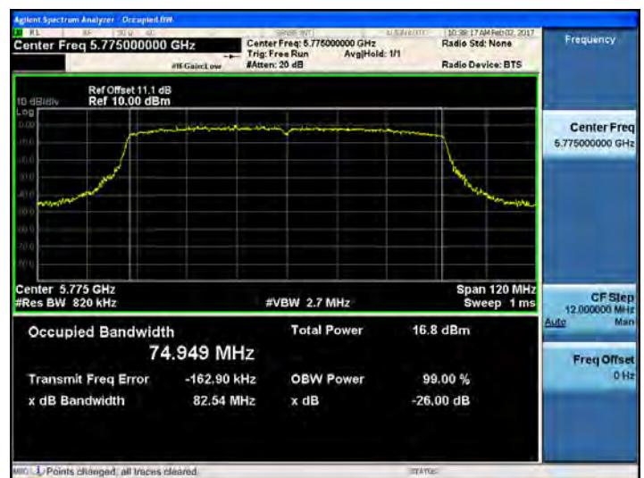
802.11ac_VHT80 UNII 3 BAND 26dB Bandwidth(CH 155)
