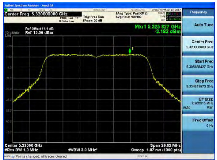
802.11ac_VHT20 UNII 3 BAND PSD CH 149
