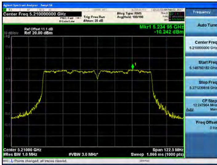
802.11ac_VHT80 UNII 2C BAND PSD CH 106
