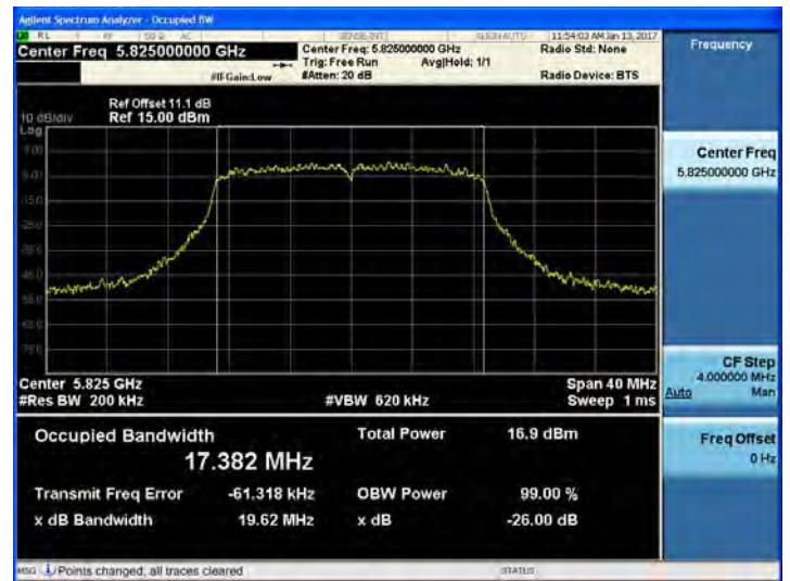
802.11ac_VHT20 UNII 3 BAND 26dB Bandwidth(CH 165)
