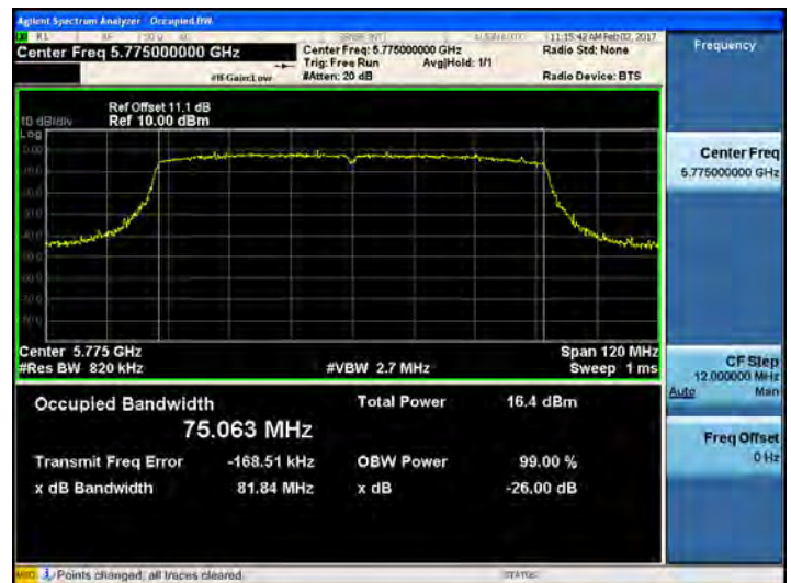
802.11ac_VHT80 UNII 3 BAND 26dB Bandwidth(CH 155)
