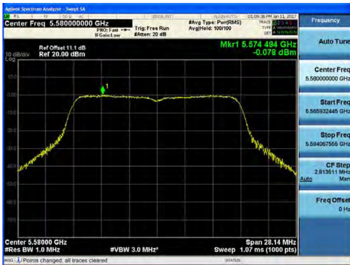
802.11a UNII 2C BAND PSD CH 116
