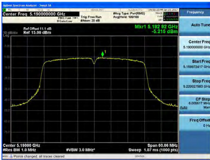
802.11n_HT40 UNII 2C BAND PSD CH 102
