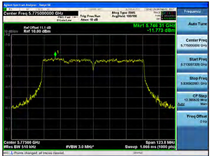
802.11ac_VHT80 UNII 3 BAND PSD CH 155
