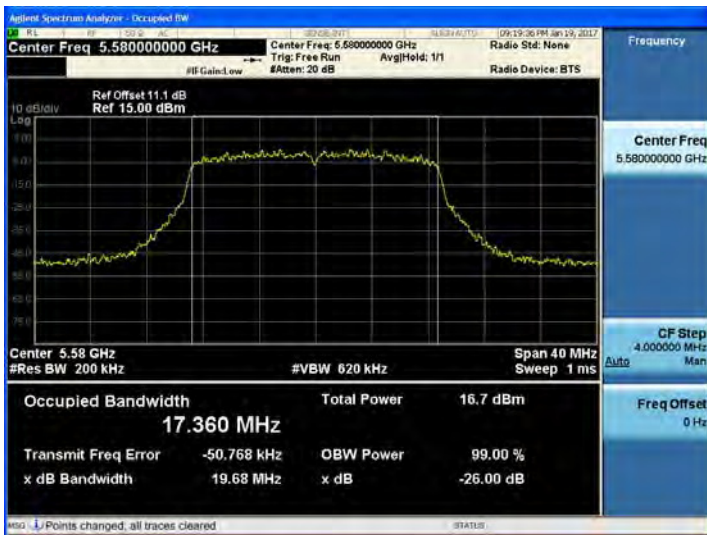
802.11ac_VHT20 UNII 2C BAND 26dB Bandwidth(CH 116)
