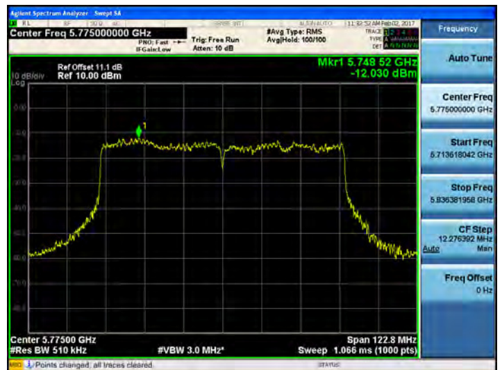
802.11ac_VHT80 UNII 3 BAND PSD CH 155
