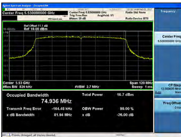
802.11ac_VHT80 UNII 2C BAND 26dB Bandwidth(CH 106)
