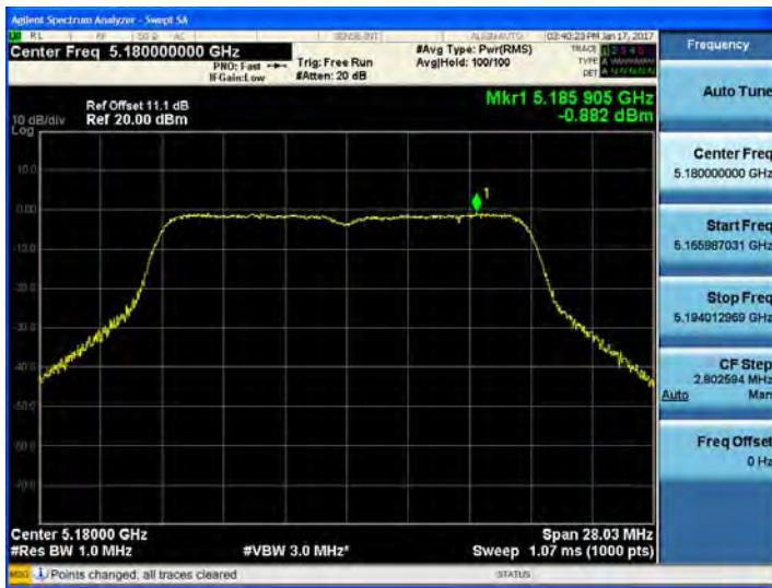
802.11a UNII 2C BAND PSD CH 116
