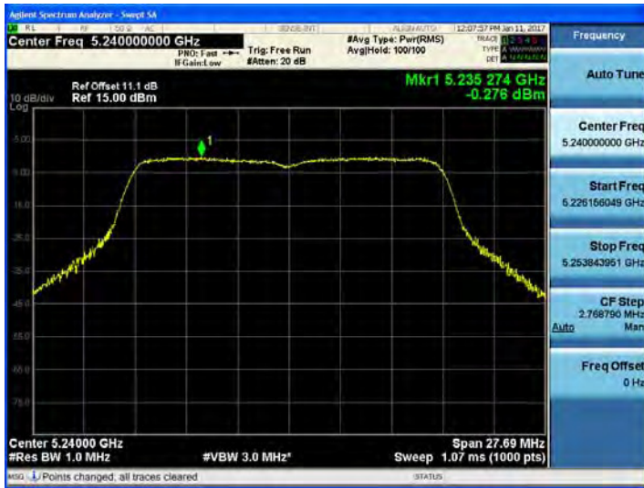
802.11a UNII 2C BAND PSD CH 116
