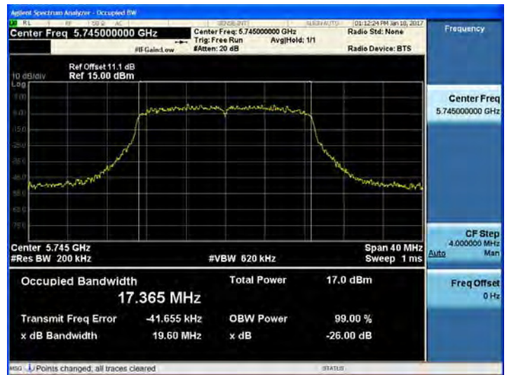
802.11n_HT20 UNII 3 BAND 26dB Bandwidth(CH 149)
