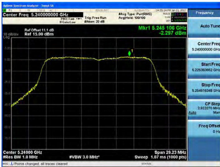
802.11n_HT20 UNII 2C BAND PSD CH 116
