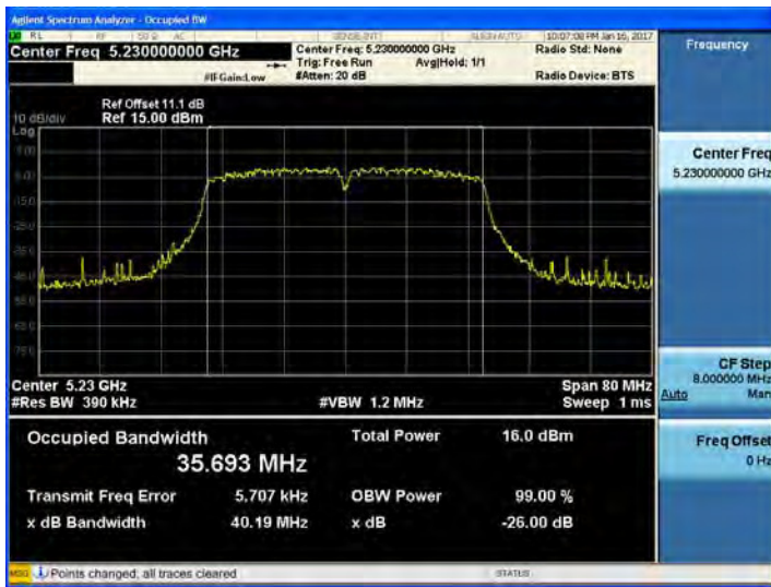
802.11ac_VHT40 UNII 2C BAND 26dB Bandwidth(CH 102)
