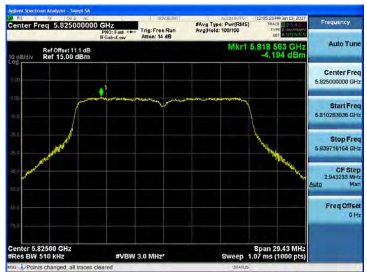
802.11ac_VHT20 UNII 3 BAND PSD CH 165
