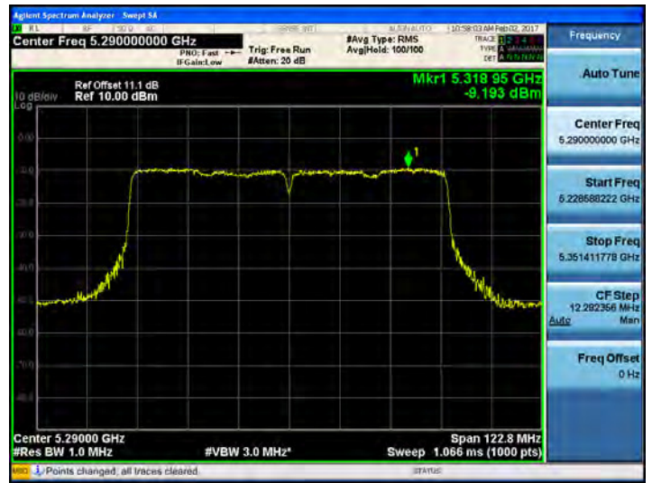
802.11ac_VHT80 UNII 3 BAND PSD CH 155
