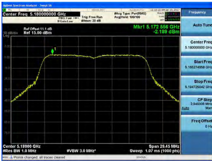
802.11ac_VHT20 UNII 2C BAND PSD CH 116
