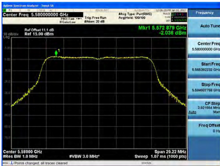
802.11n_HT20 UNII 2C BAND PSD CH 116
