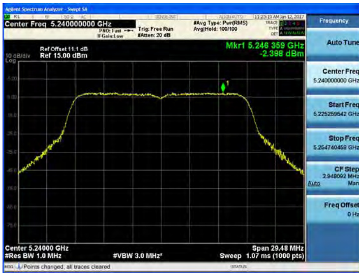
802.11ac_VHT20 UNII 2C BAND PSD CH 116
