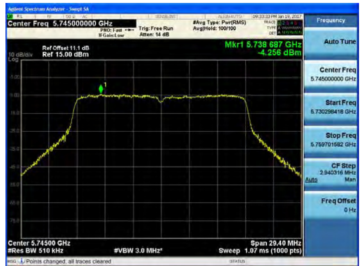
802.11ac_VHT20 UNII 3 BAND PSD CH 149
