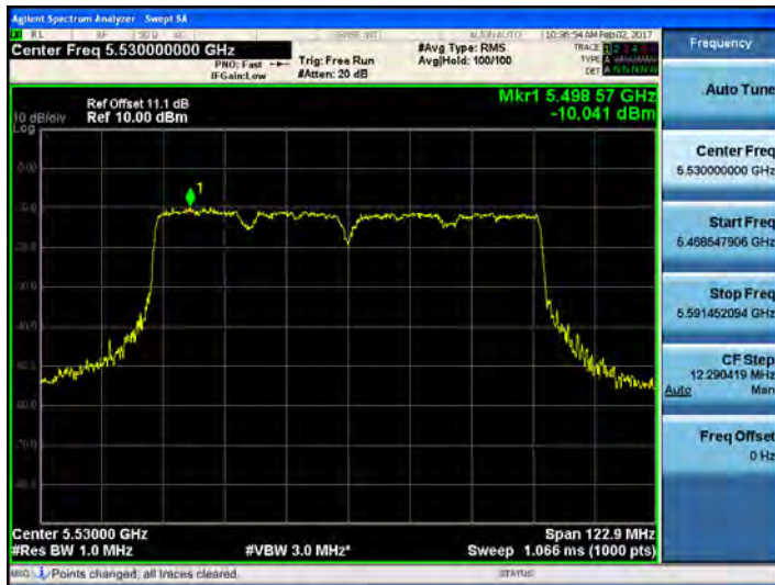
802.11ac_VHT80 UNII 2C BAND PSD CH 106
