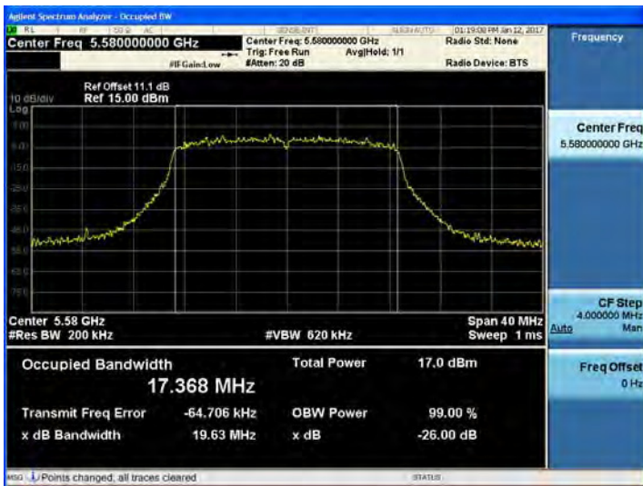
802.11ac_VHT20 UNII 2C BAND 26dB Bandwidth(CH 116)
