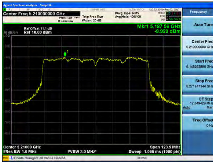
802.11ac_VHT80 UNII 2C BAND PSD CH 106
