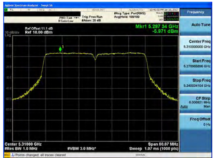
802.11ac_VHT40 UNII 3 BAND PSD CH 151
