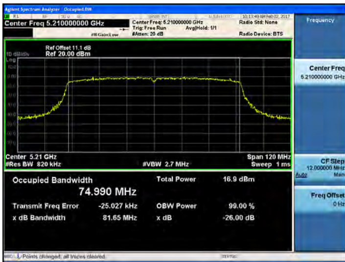
802.11ac_VHT80 UNII 2C BAND 26dB Bandwidth(CH 106)
