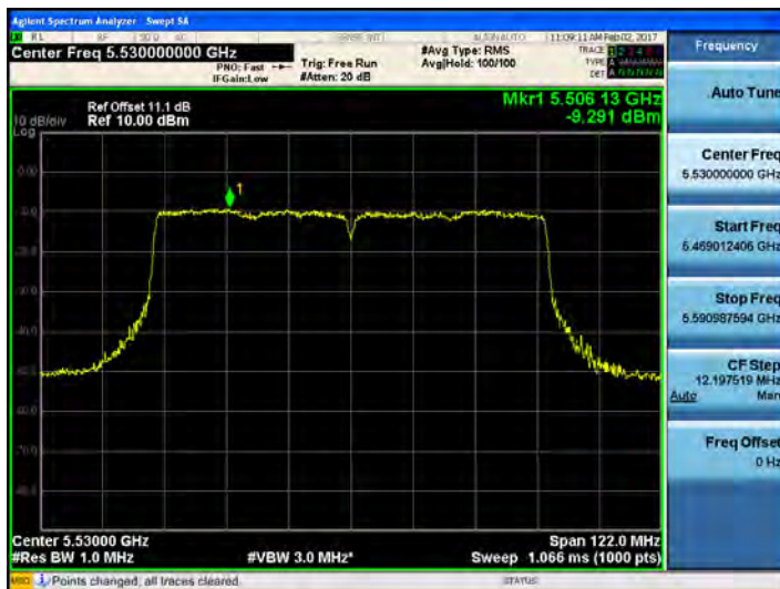
802.11ac_VHT80 UNII 2C BAND PSD CH 106
