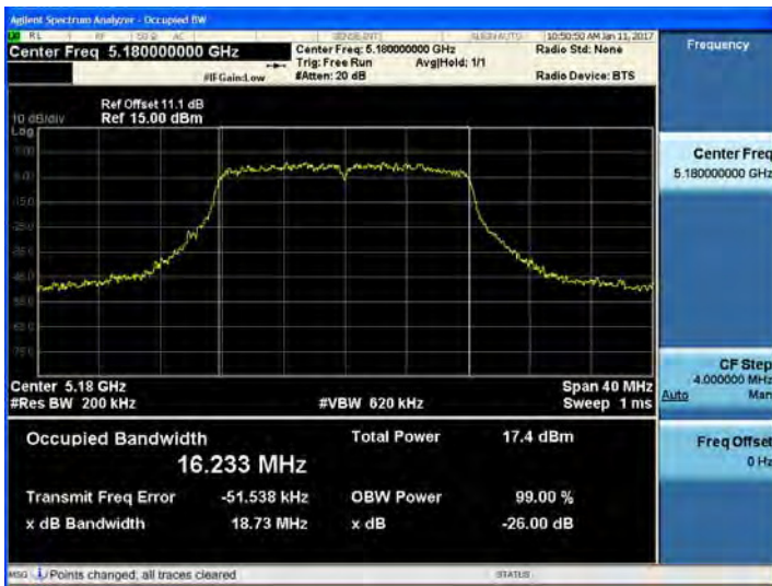
802.11a UNII 2C BAND 26dB Bandwidth (CH116)
