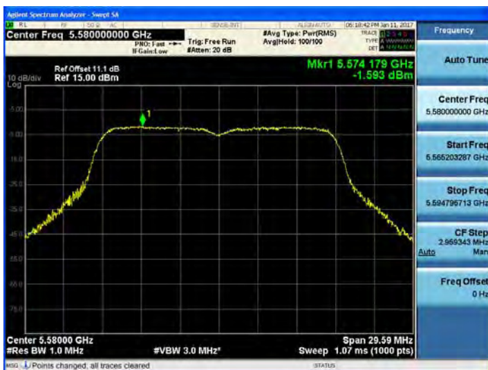
802.11n_HT20 UNII 2C BAND PSD CH 116
