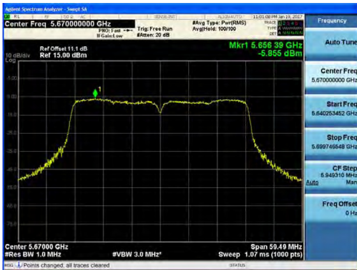
802.11ac_VHT40 UNII 2C BAND PSD CH 134
