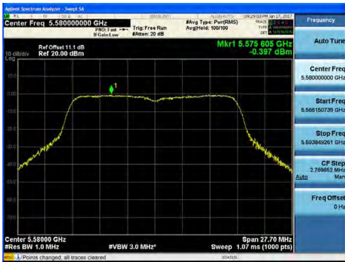
802.11a UNII 2C BAND PSD CH 116
