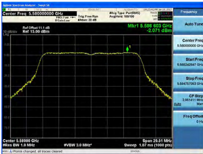
802.11ac_VHT20 UNII 2C BAND PSD CH 116
