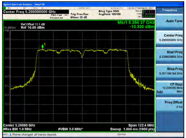
802.11ac_VHT80 UNII 3 BAND PSD CH 155
