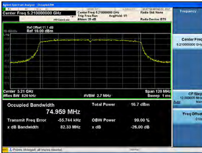
802.11ac_VHT80 UNII 2C BAND 26dB Bandwidth(CH 106)
