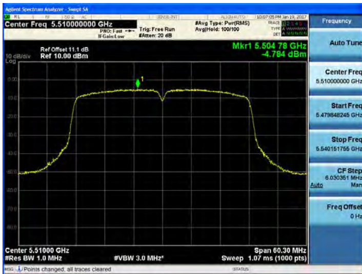
802.11n_HT40 UNII 2C BAND PSD CH 102
