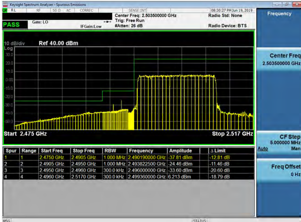
Plot 7-234. Lower ACP Plot (Band 41 - 15.0MHz QPSK - Full RB Configuration)
