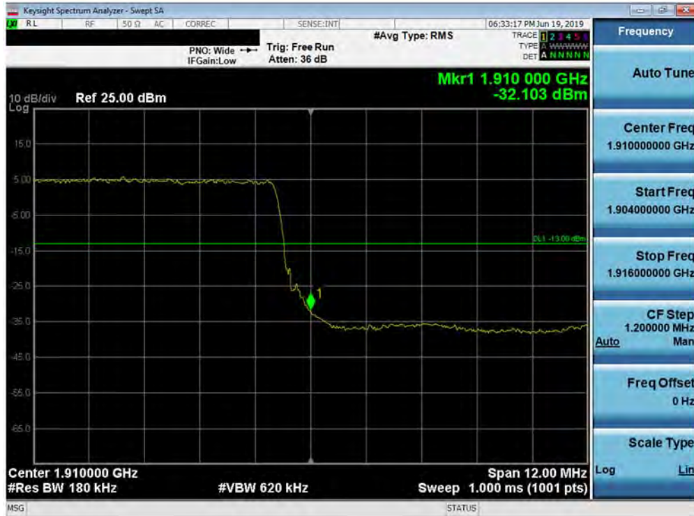
Plot 7-220. Upper Band Edge Plot (Band 2 - 15.0MHz QPSK - Full RB Configuration)
