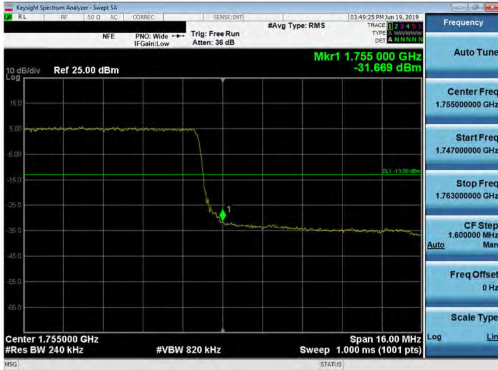
Plot 7-190. Upper Band Edge Plot (Band 4 - 20.0MHz QPSK - Full RB Configuration)
