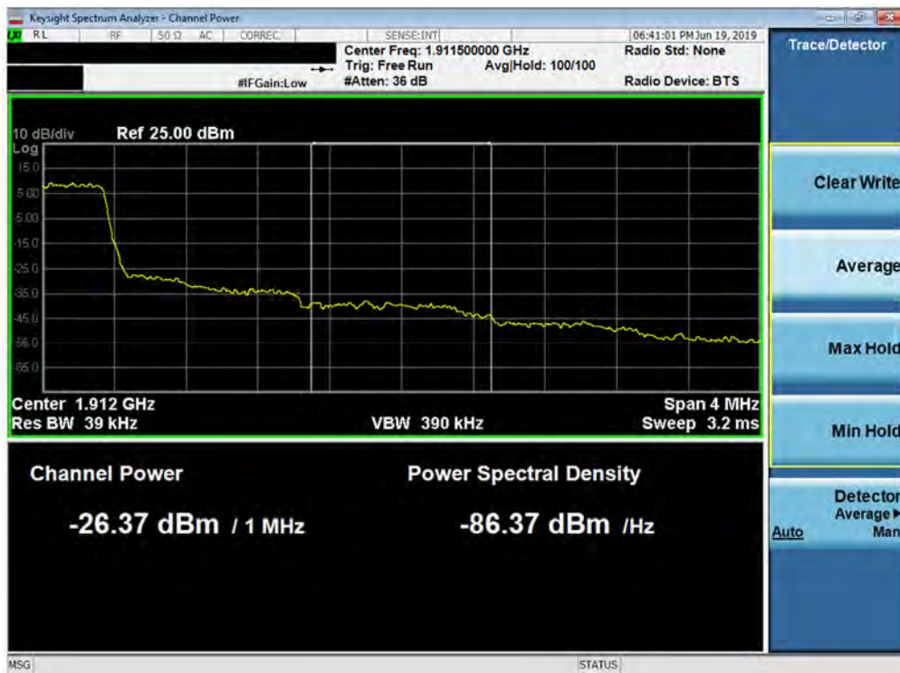
Plot 7-197. Upper Extended Band Edge Plot (Band 2 - 1.4MHz QPSK - Full RB Configuration)
