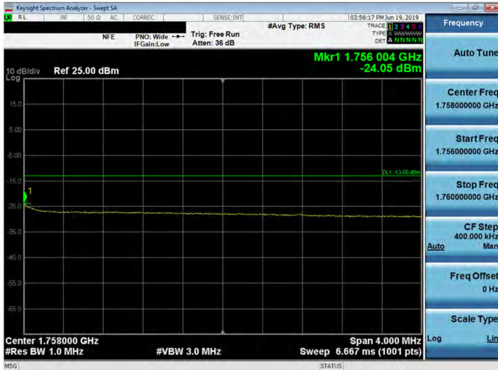
Plot 7-179. Upper Extended Band Edge Plot (Band 4 - 10.0MHz QPSK - Full RB Configuration)
