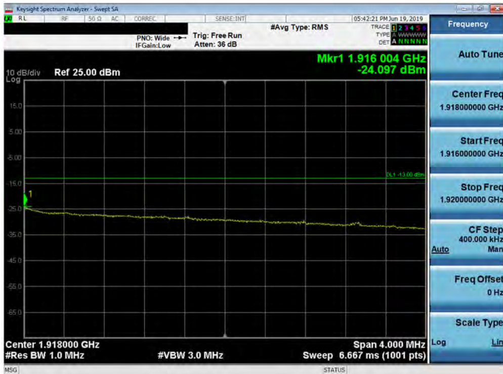
Plot 7-217. Upper Extended Band Edge Plot (Band 25 - 10.0MHz QPSK - Full RB Configuration)
