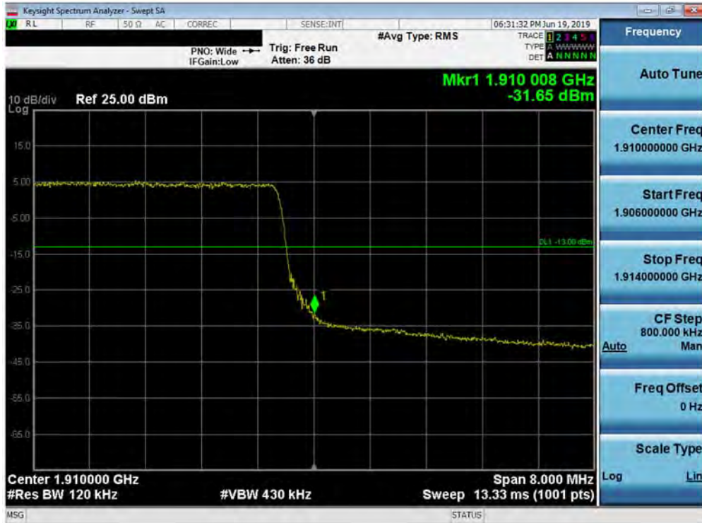
Plot 7-214. Upper Band Edge Plot (Band 2 - 10.0MHz QPSK - Full RB Configuration)
