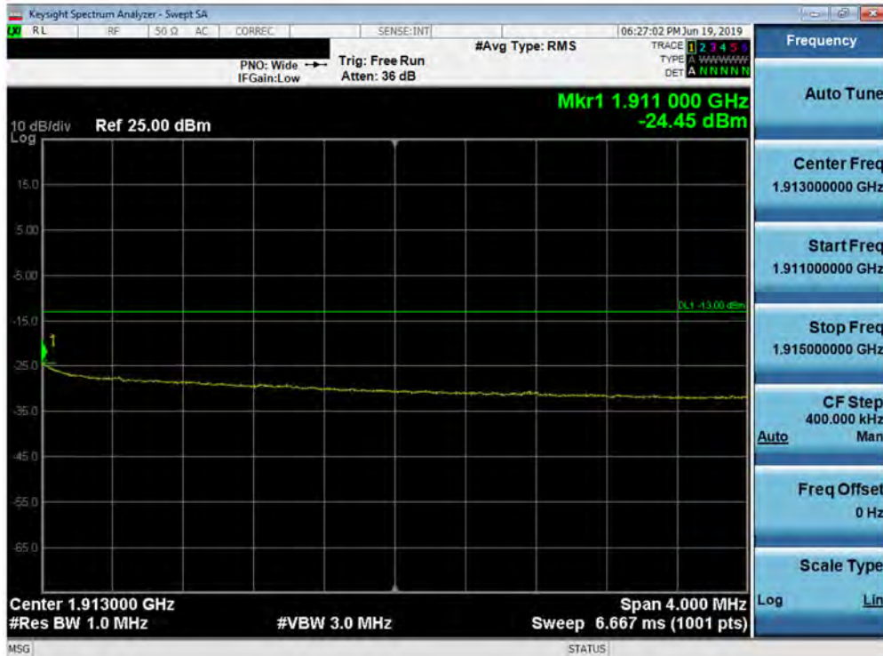
Plot 7-215. Upper Extended Band Edge Plot (Band 2 - 10.0MHz QPSK - Full RB Configuration)
