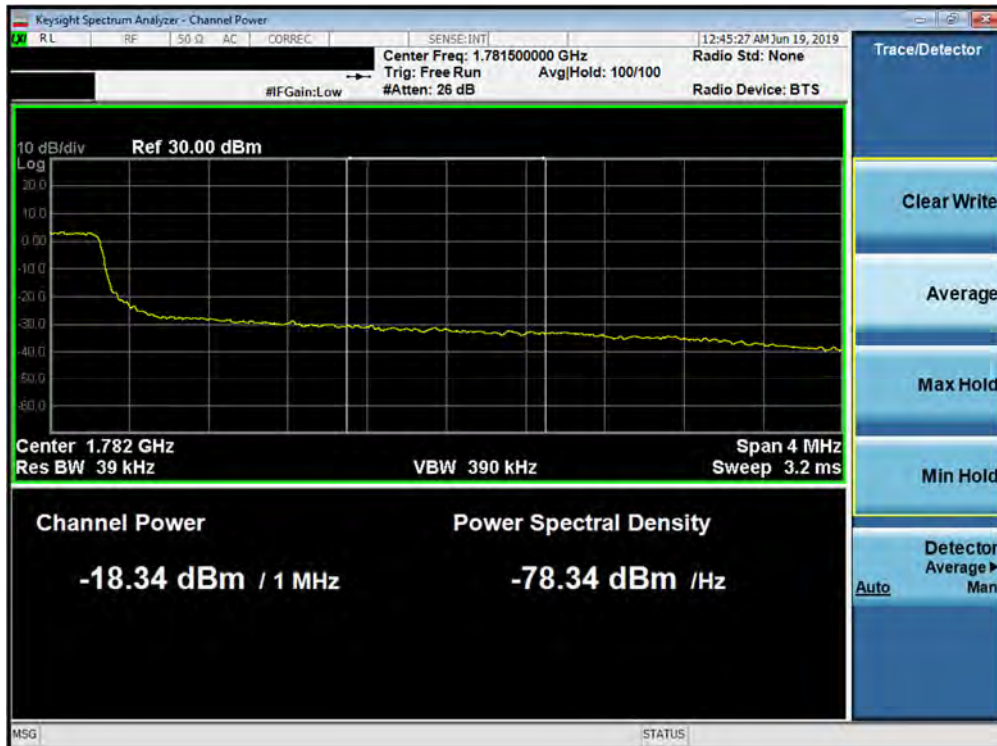
Plot 7-175. Upper Extended Band Edge Plot (Band 66 - 5.0MHz QPSK - Full RB Configuration)
