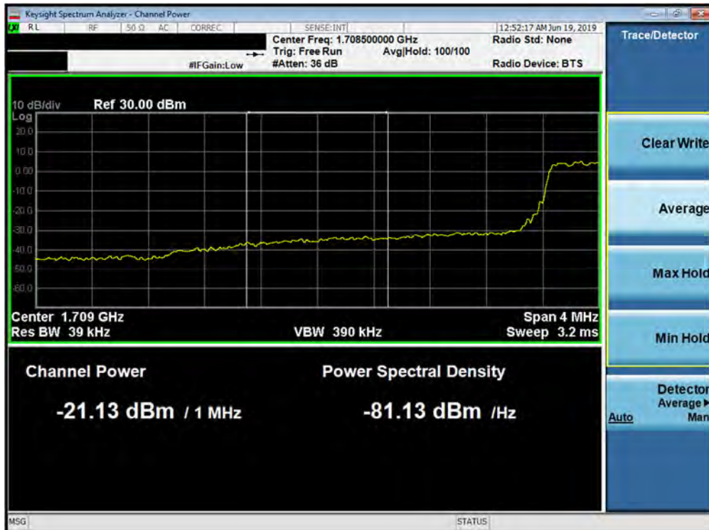
Plot 7-165. Lower Extended Band Edge Plot (Band 66/4 - 3.0MHz QPSK - Full RB Configuration)
