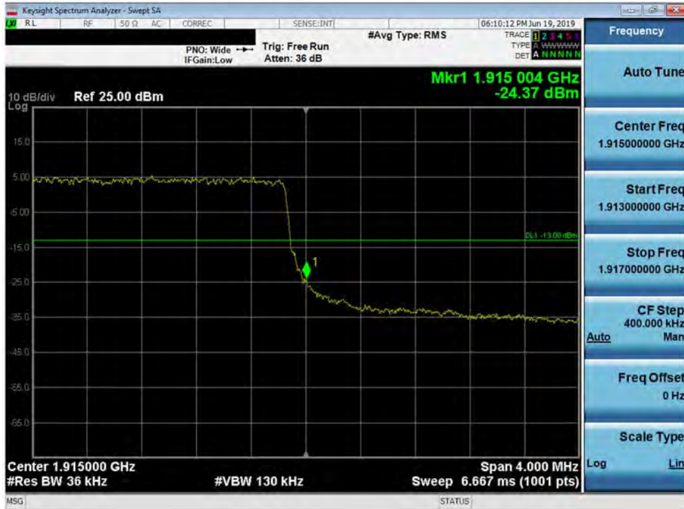
Plot 7-204. Upper Band Edge Plot (Band 25 - 3.0MHz QPSK - Full RB Configuration)
