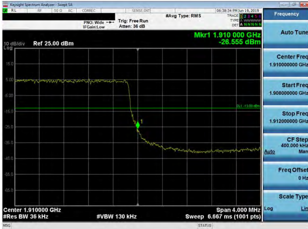
Plot 7-202. Upper Band Edge Plot (Band 2 - 3.0MHz QPSK - Full RB Configuration)
