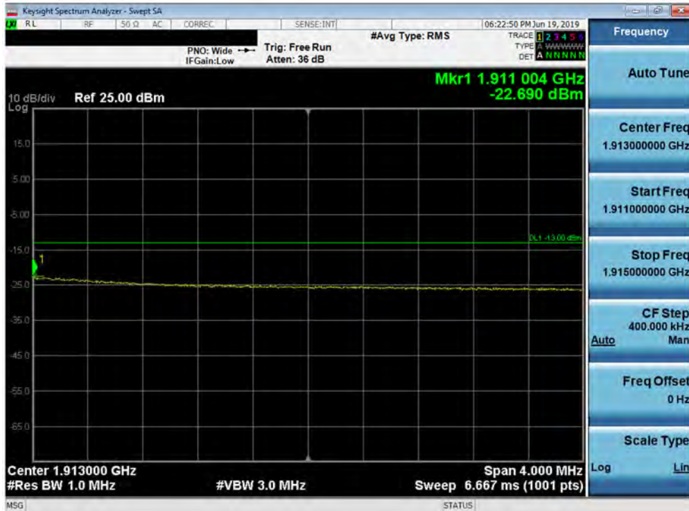
Plot 7-227. Upper Extended Band Edge Plot (Band 2 - 20.0MHz QPSK - Full RB Configuration)
