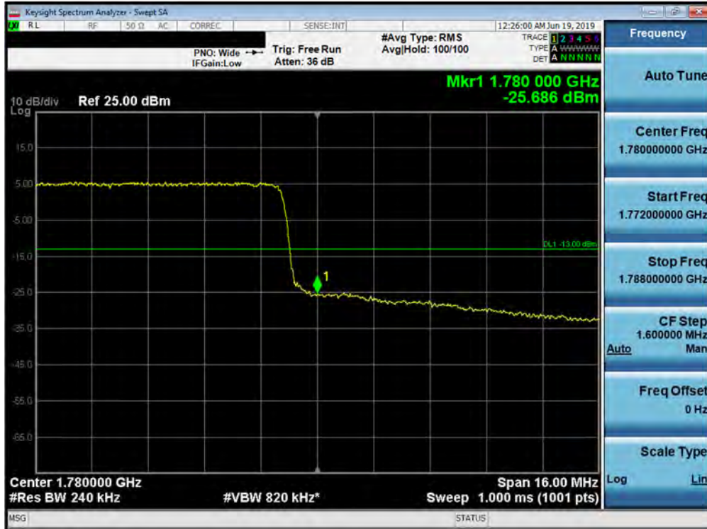
Plot 7-192. Upper Band Edge Plot (Band 66 - 20.0MHz QPSK - Full RB Configuration)
