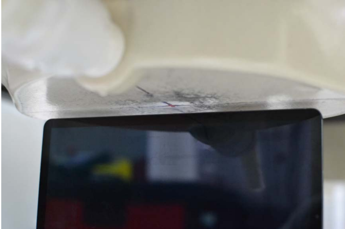
SAR Test Setup Photo 9 – Left Edge at 0.6 cm
