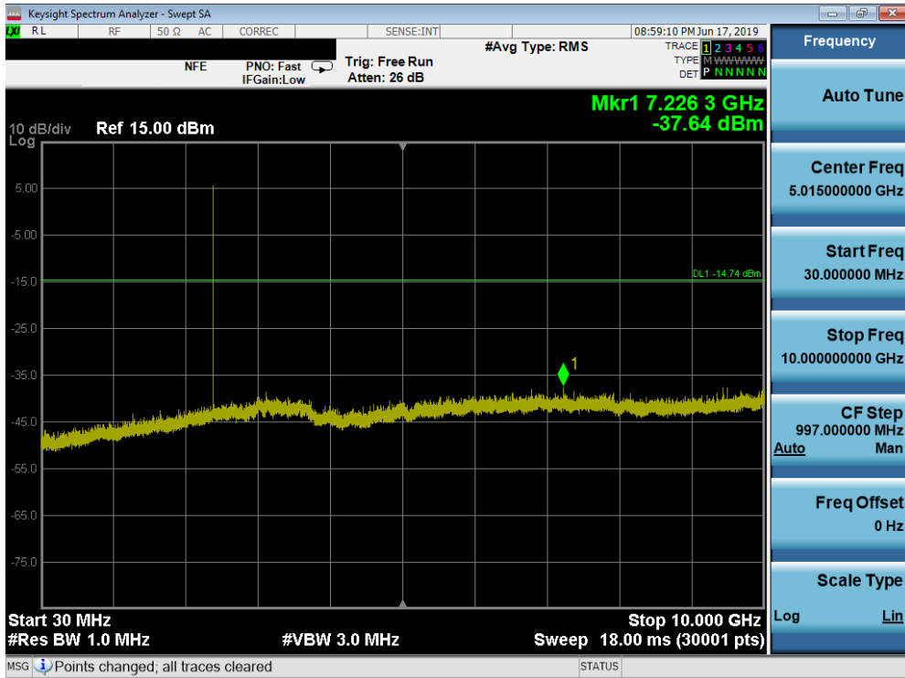
Plot 7-39. Conducted Spurious Plot (Bluetooth (LE), 2Mbps – Ch. 0)
