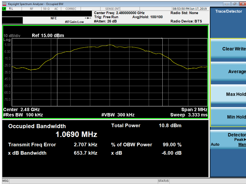
Plot 7-9. 6dB Bandwidth Plot (Bluetooth (LE), 1Mbps – Ch. 39)
