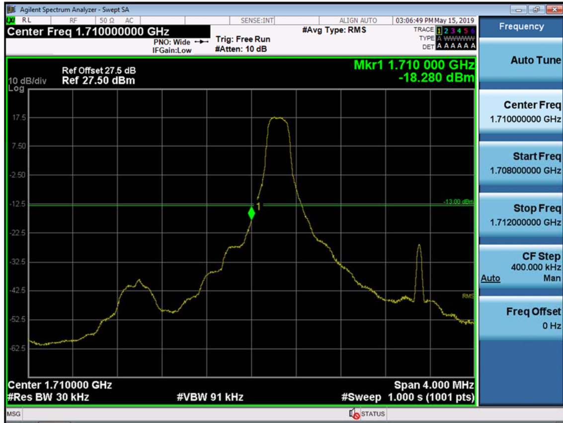
BAND 66/4. Lower Band Edge Plot (3M BW Ch.131987 QPSK RB 1, Offset 0) -1
