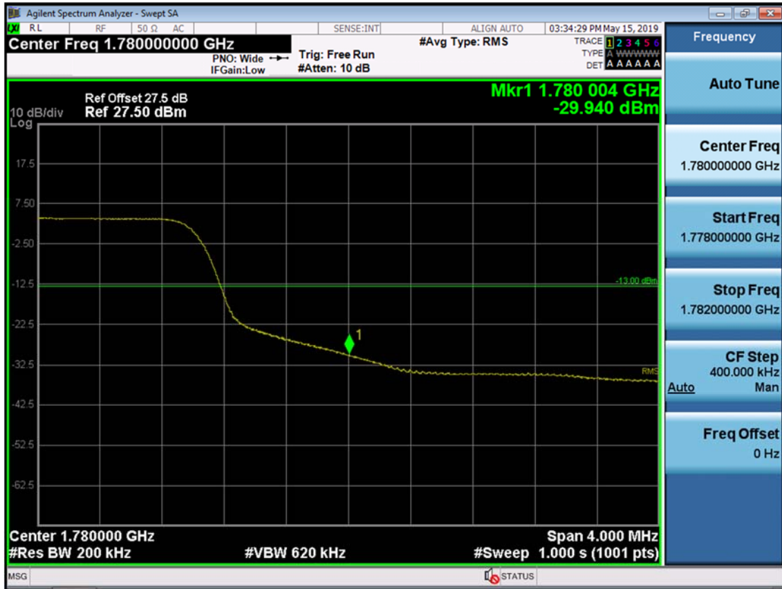
BAND 66/4. Upper Band Edge Plot (20M BW Ch.132572 QPSK_RB100) -2
