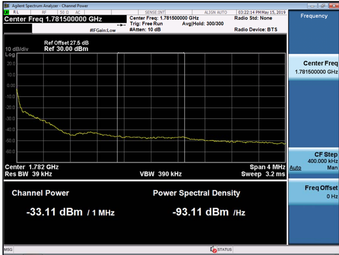
BAND 66/4. Upper Extended Band Edge Plot (10M BW Ch.132622 QPSK_RB50) -3
