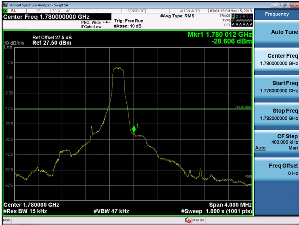
BAND 66/4. Upper Band Edge Plot (1.4M BW Ch.132665 QPSK_RB1_Offset 5) -1
