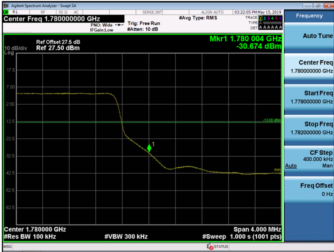
BAND 66/4. Upper Band Edge Plot (10M BW Ch.132622 QPSK_RB50) -2
