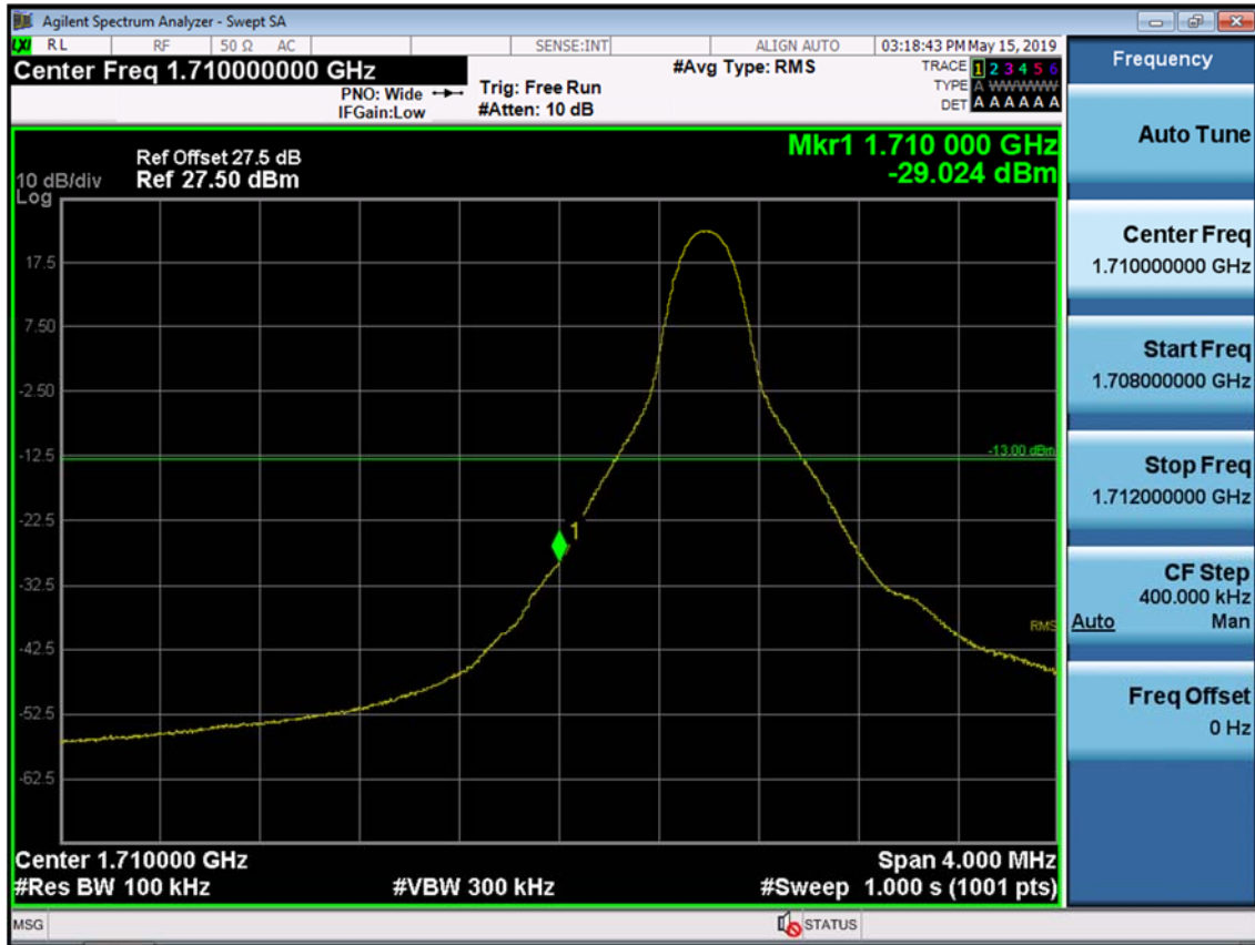
BAND 66/4. Lower Band Edge Plot (10M BW Ch.132022 QPSK RB 1, Offset 0) -1
