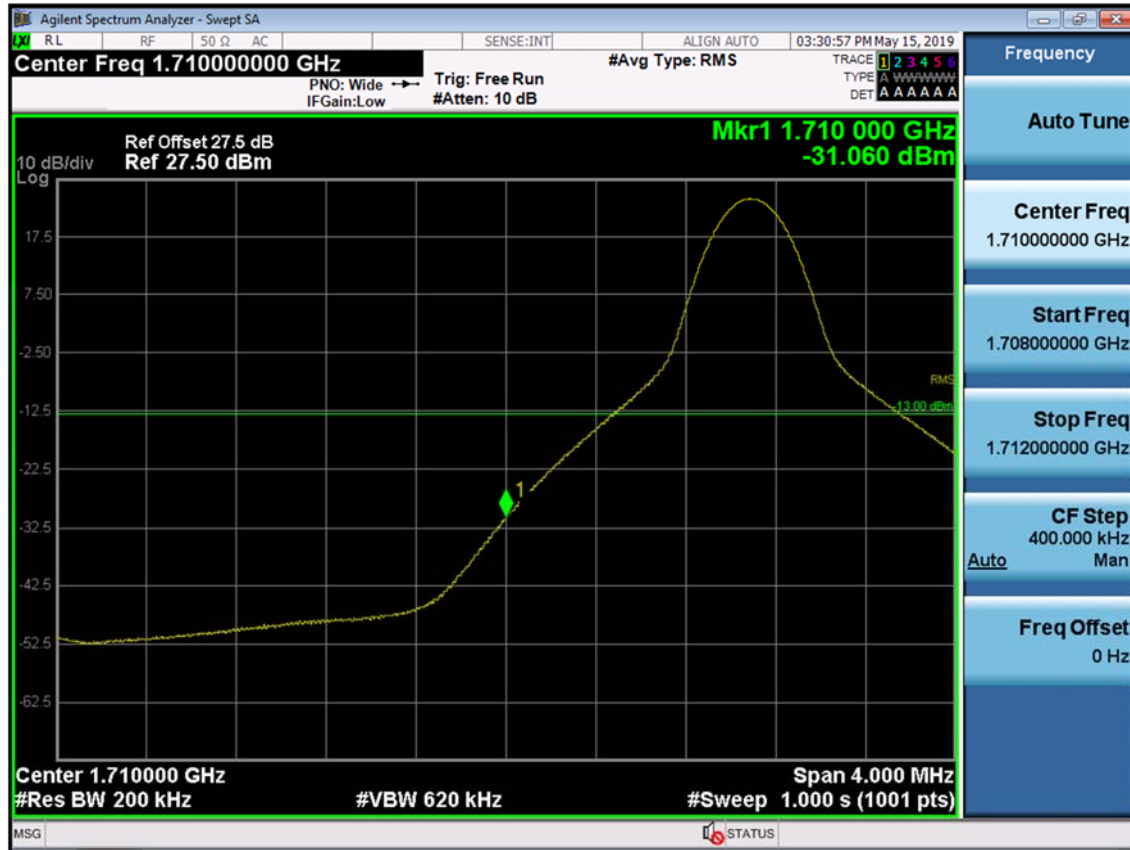
BAND 66/4. Lower Band Edge Plot (20M BW Ch.132072 QPSK RB 1, Offset 0) -1
