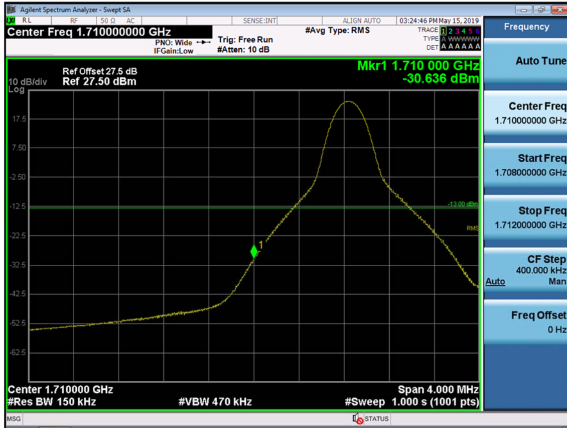
BAND 66/4. Lower Band Edge Plot (15M BW Ch.132047 QPSK RB 1, Offset 0) -1
