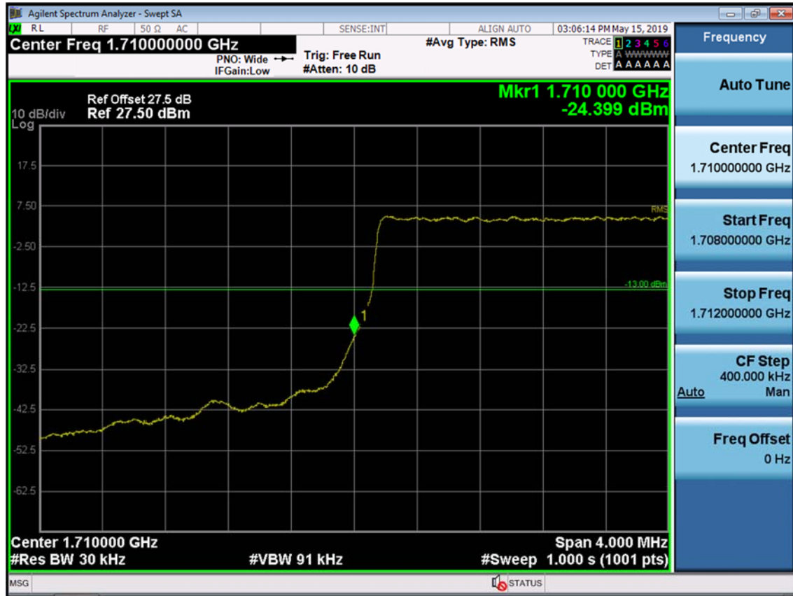
BAND 66/4. Lower Band Edge Plot (3M BW Ch.131987 QPSK RB 15) -2
