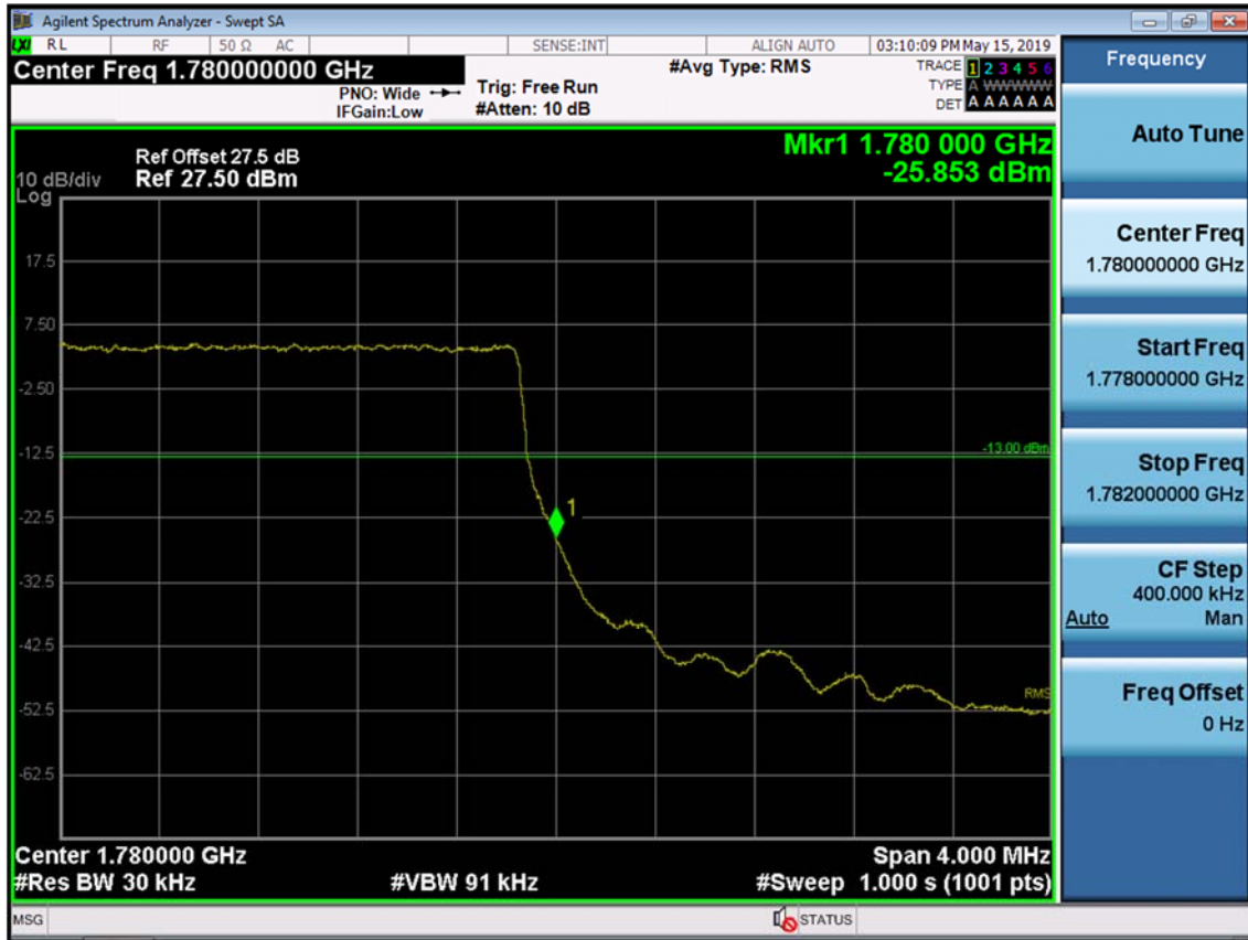
BAND 66/4. Upper Band Edge Plot (3M BW Ch.132657 QPSK_RB15) -2
