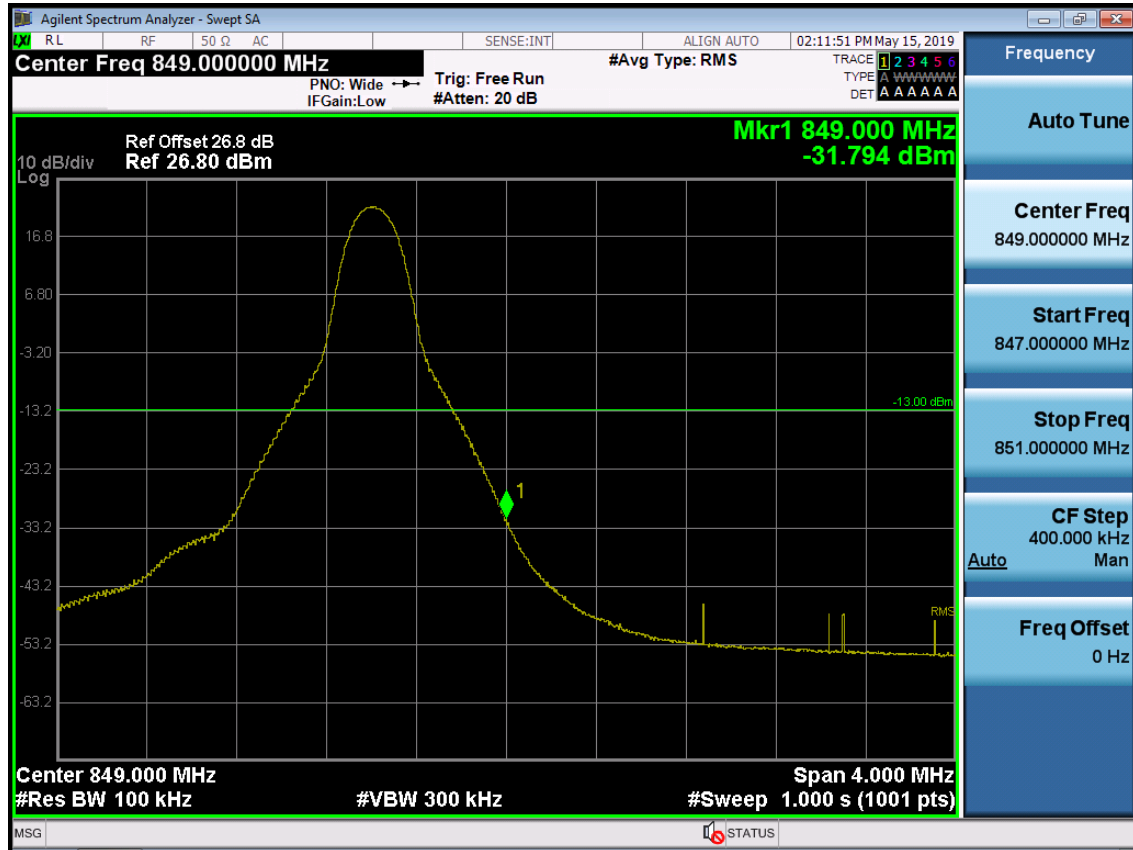
BAND 5. Upper Band Edge Plot (10M BW Ch.20600 QPSK_RB1_Offset 49)
