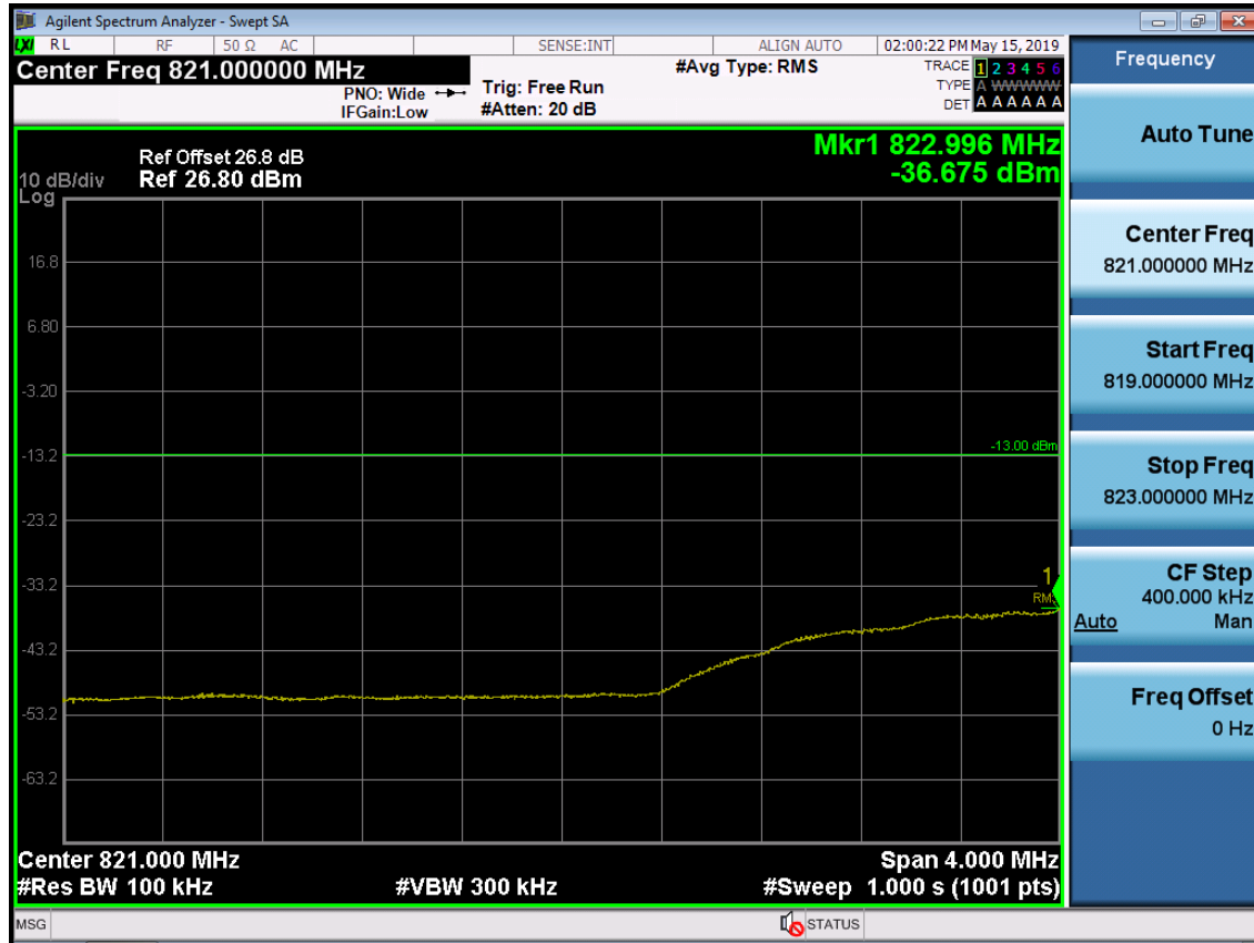
BAND 5. Lower Extended Band Edge Plot (3M BW Ch.20415 QPSK_RB15_0)
