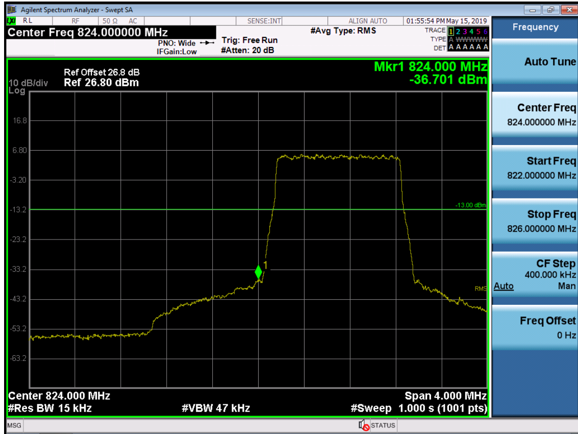
BAND 5. Lower Band Edge Plot (1.4M BW Ch.20407 QPSK_RB6_Offset 0)
