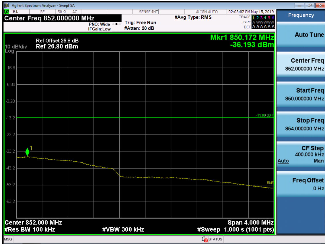
BAND 5. Upper Extended Band Edge Plot (3M BW Ch.20635 QPSK_RB15_0)
