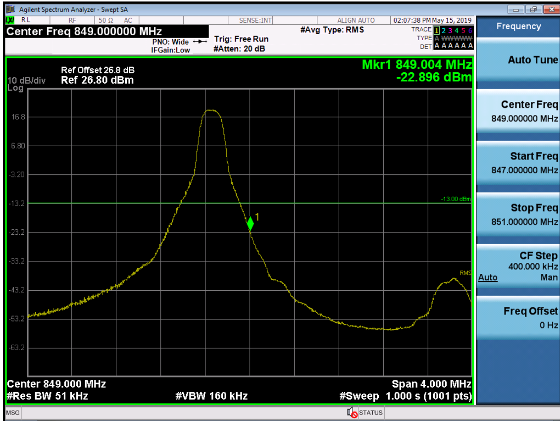
BAND 5. Upper Band Edge Plot (5M BW Ch.20625 QPSK_RB1_Offset 24)
