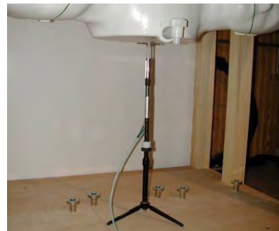
Figure 10-2 System Verification Setup Photo
