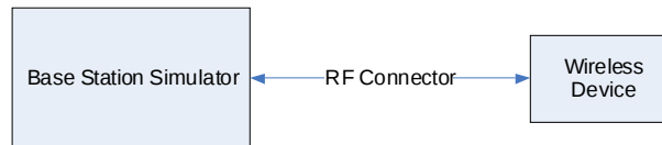
Figure 9-1 Power Measurement Setup
