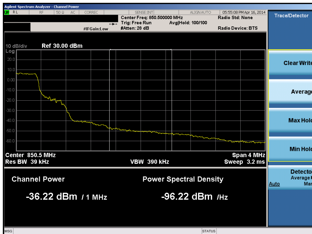
Plot 6-18. Upper Extended Band Edge Plot (Band 5 – 1.4MHz QPSK – RB Size 6)
