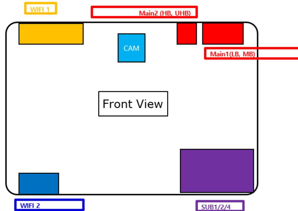
※ Coaxial cables are connected to each antenna.
