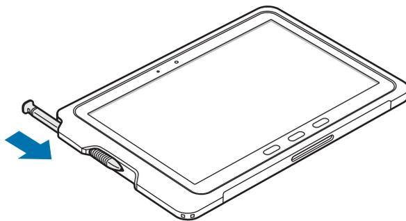
**!** Do not insert the S Pen backwards into the protective case.
