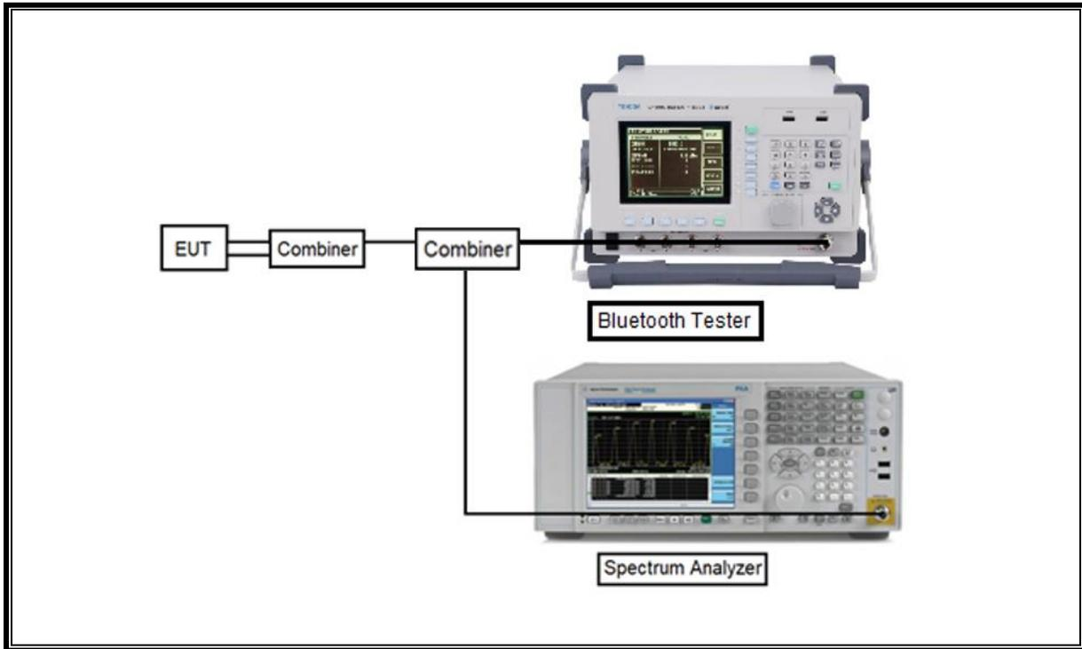
**SETUP DIAGRAM FOR TESTS (RADIATED TEST SETUP)**
