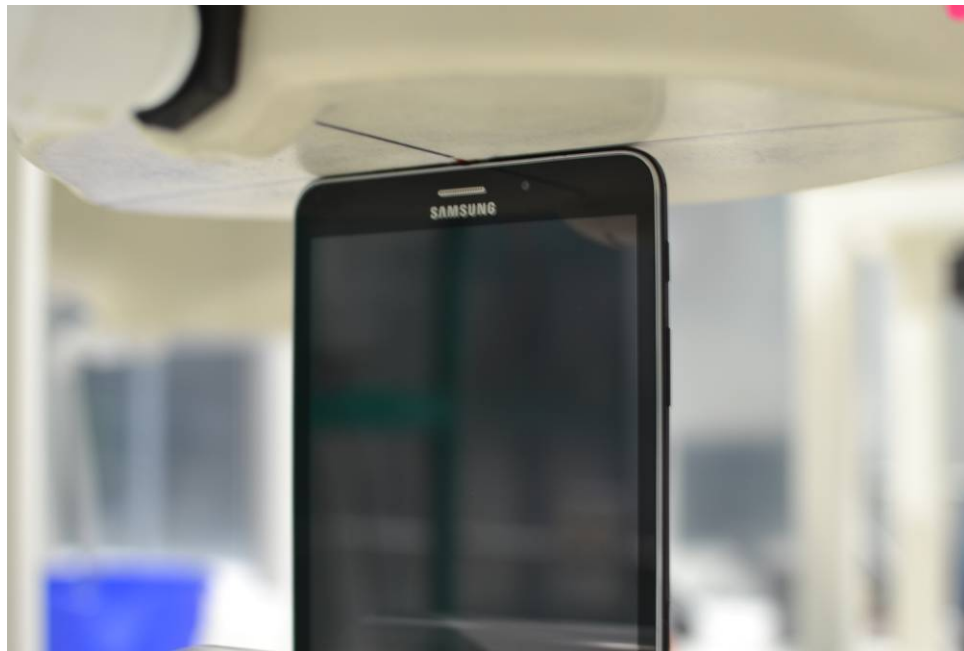
SAR Test Setup Photo 8: Top Edge at 0 mm
