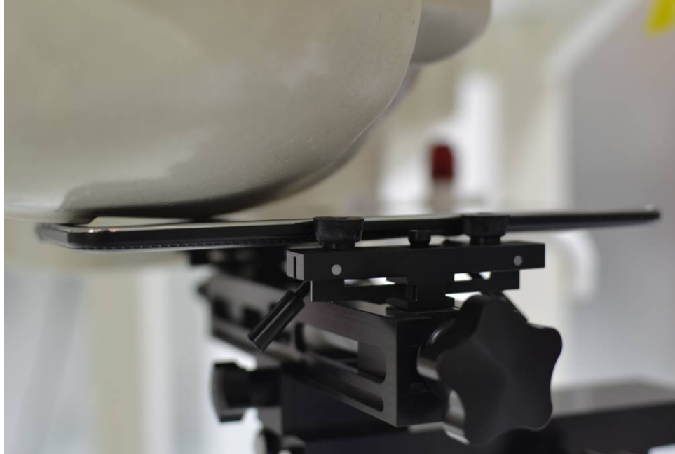
SAR Test Setup Photo 1: Right Cheek
