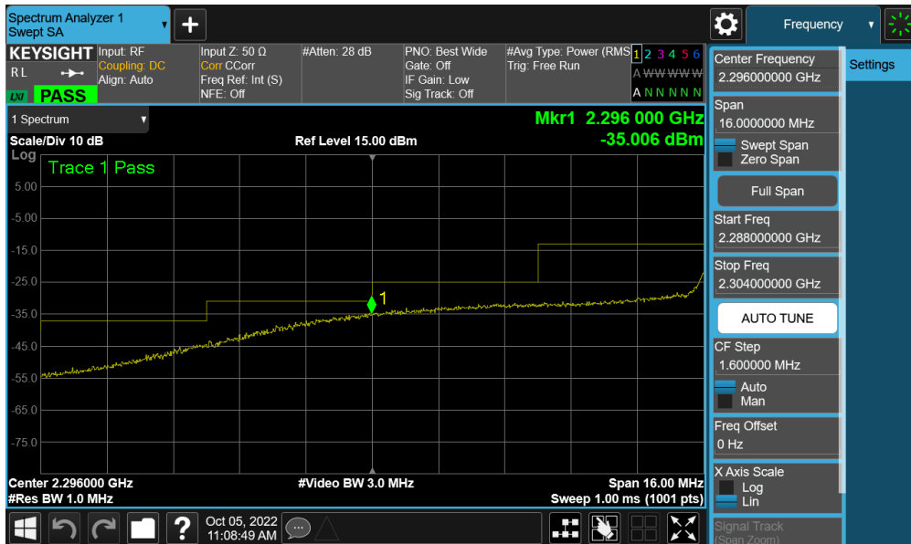
Plot 7-383. Extended Lower Band Edge Plot (NR Band n30 - 10MHz CP-OFDM-QPSK – Full RB - Ant F)
