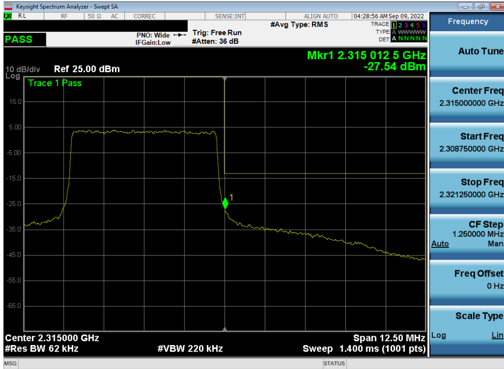
Plot 7-332. Upper Band Edge Plot (LTE Band 30 - 5MHz QPSK – Full RB - Ant A)
