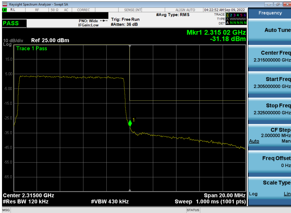
Plot 7-328. Upper Band Edge Plot (LTE Band 30 - 10MHz QPSK – Full RB - Ant A)
