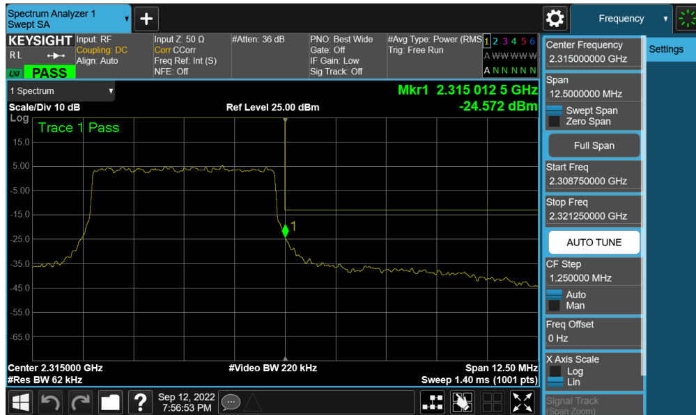
Plot 7-380. Upper Band Edge Plot (NR Band n30 - 5MHz CP-OFDM-QPSK – Full RB - Ant A)
