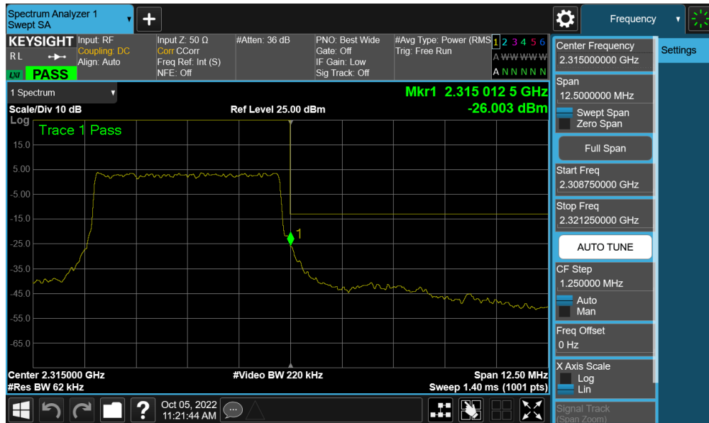
Plot 7-388. Upper Band Edge Plot (NR Band n30 - 5MHz CP-OFDM-QPSK – Full RB - Ant F)
