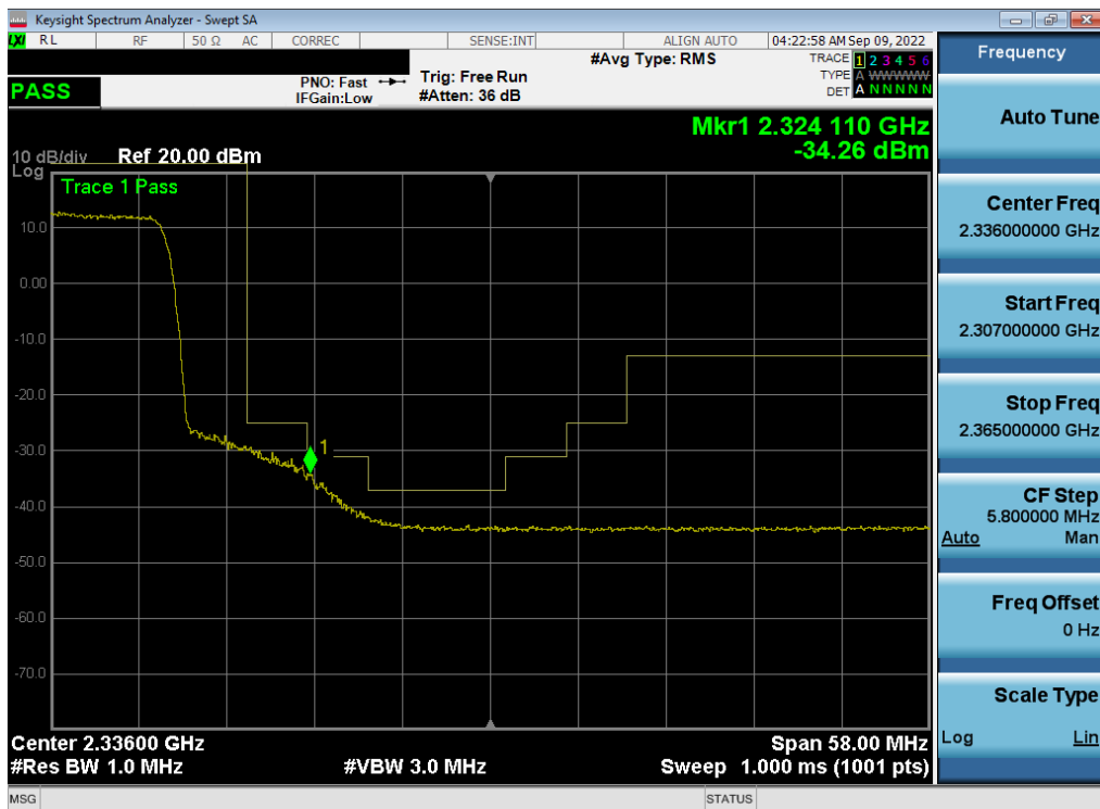
Plot 7-329. Extended Upper Band Edge Plot (LTE Band 30 - 10MHz QPSK – Full RB - Ant A)
