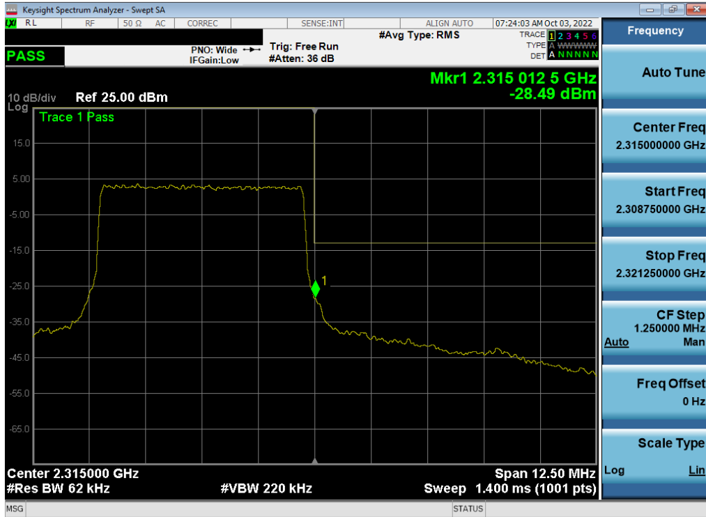
Plot 7-340. Upper Band Edge Plot (LTE Band 30 - 5MHz QPSK – Full RB - Ant F)
