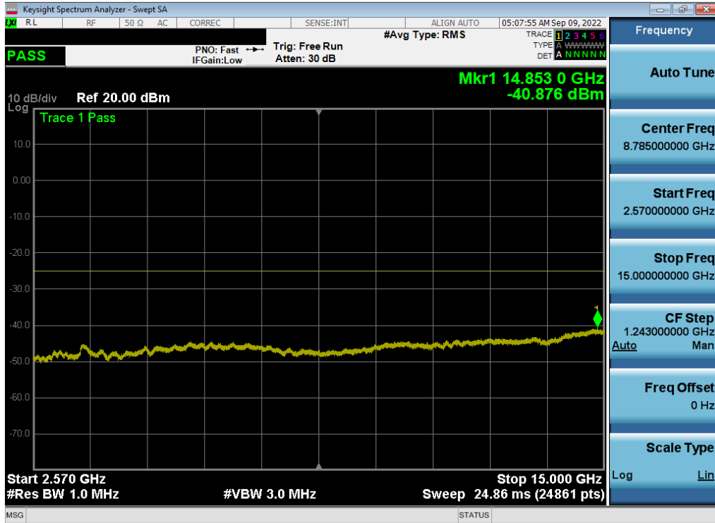
Plot 7-171. Conducted Spurious Plot (LTE Band 7 - 20MHz QPSK - RB Size 1, RB Offset 0 - Mid Channel - Ant B)
