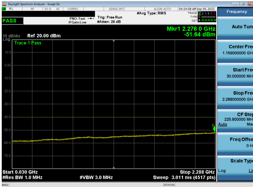
Plot 7-161. Conducted Spurious Plot (LTE Band 30 - 10MHz QPSK - RB Size 1, RB Offset 0 - Ant A)
