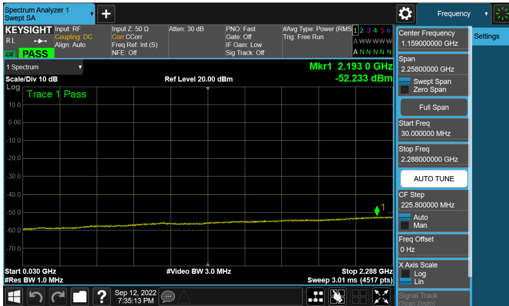
Plot 7-212. Conducted Spurious Plot (NR Band n30 - 10MHz QPSK - RB Size 1, RB Offset 0 – Ant A)
