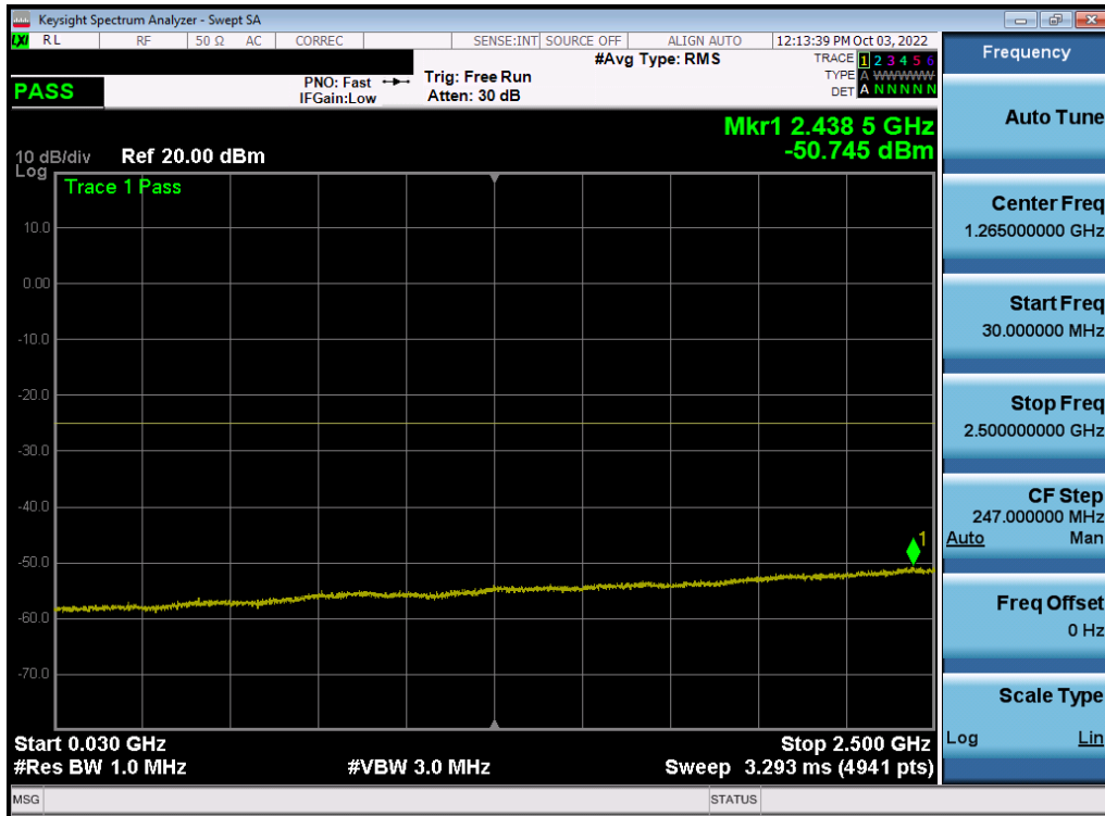
Plot 7-182. Conducted Spurious Plot (LTE Band 7 - 20MHz QPSK - RB Size 1, RB Offset 0 - High Channel - Ant F)
