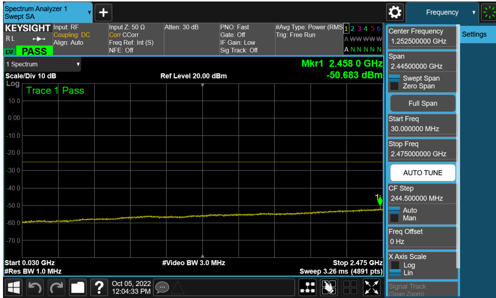
Plot 7-227. Conducted Spurious Plot (NR Band n7 - 40MHz QPSK - RB Size 1, RB Offset 0 - Low Channel Ant F)
