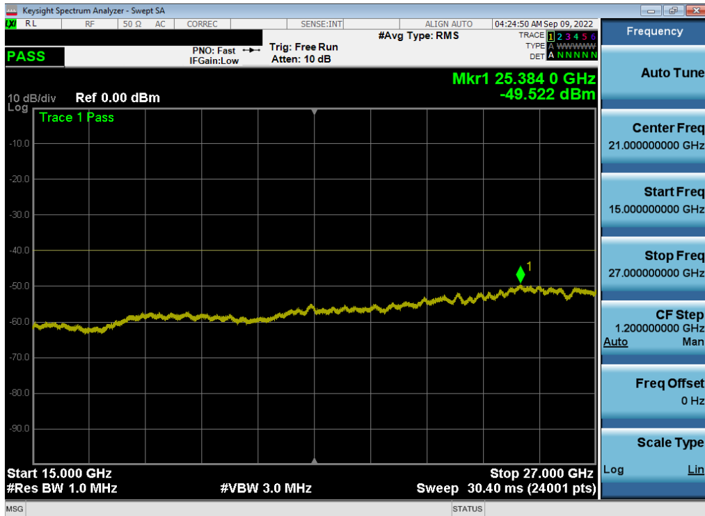
Plot 7-163. Conducted Spurious Plot (LTE Band 30 - 10MHz QPSK - RB Size 1, RB Offset 0 - Ant A)
