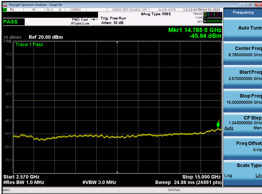
Plot 7-180. Conducted Spurious Plot (LTE Band 7 - 20MHz QPSK - RB Size 1, RB Offset 0 - Mid Channel - Ant F)
