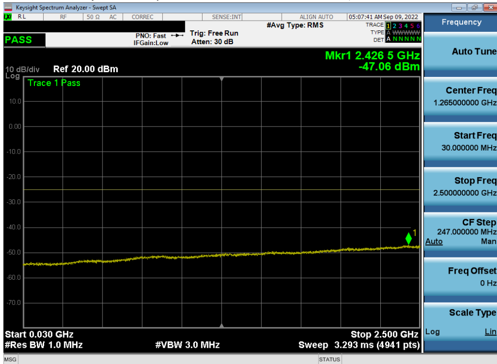
Plot 7-170. Conducted Spurious Plot (LTE Band 7 - 20MHz QPSK - RB Size 1, RB Offset 0 - Mid Channel - Ant B)
