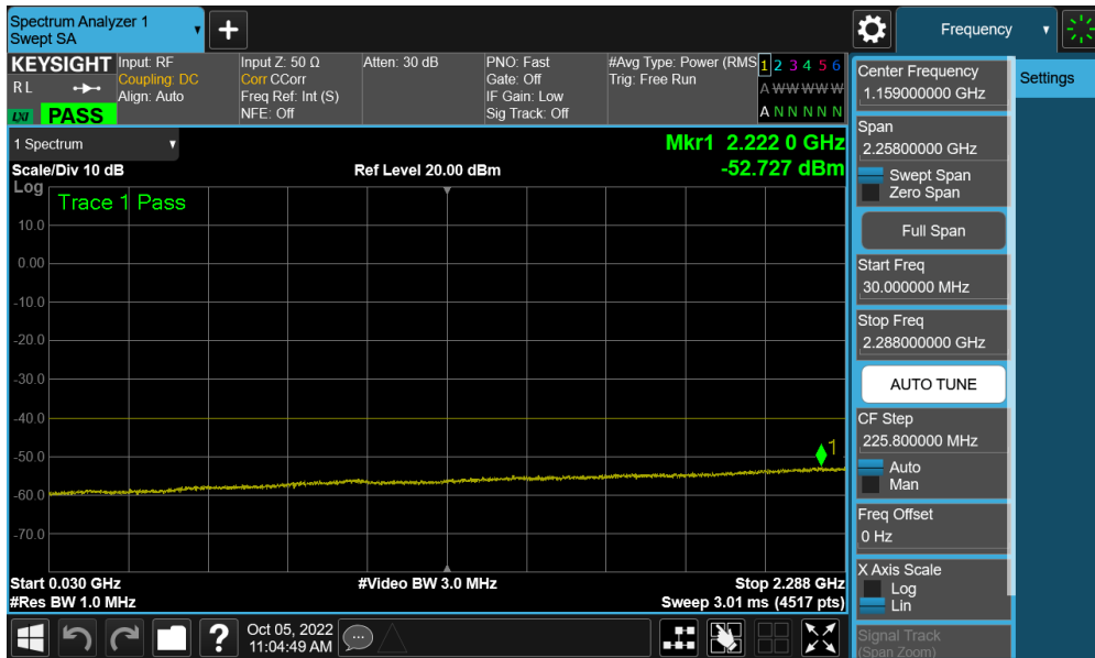
Plot 7-215. Conducted Spurious Plot (NR Band n30 - 10MHz QPSK - RB Size 1, RB Offset 0 – Ant F)
