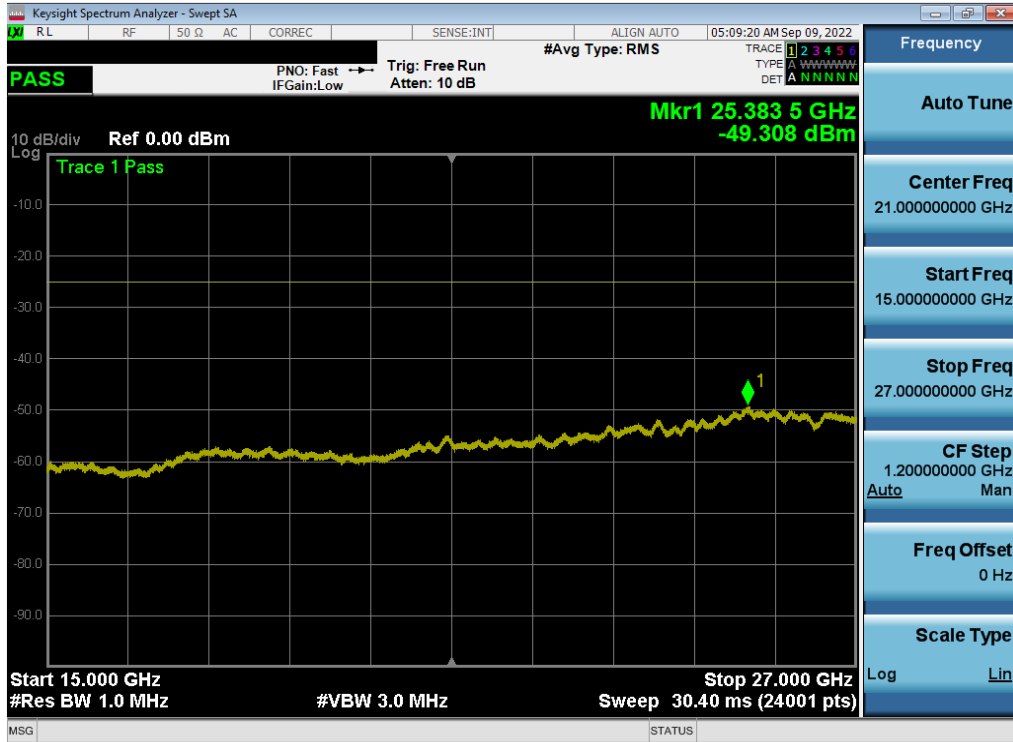
Plot 7-169. Conducted Spurious Plot (LTE Band 7 - 20MHz QPSK - RB Size 1, RB Offset 0 - Low Channel - Ant B)
