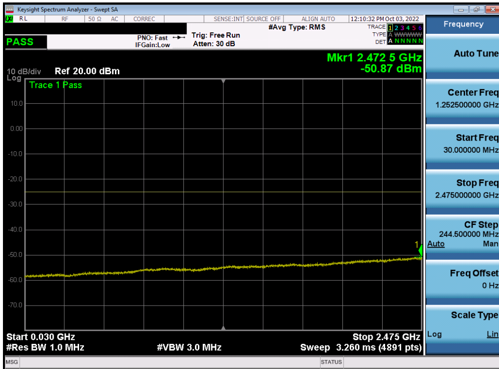
Plot 7-176. Conducted Spurious Plot (LTE Band 7 - 20MHz QPSK - RB Size 1, RB Offset 0 - Low Channel - Ant F)
