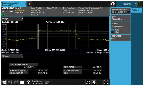
Plot 7-41. Occupied Bandwidth Plot (NR Band n30 - 10MHz π/2 BPSK - Full RB - Ant A)
