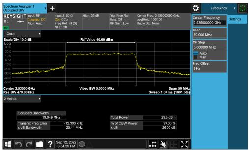
Plot 7-55. Occupied Bandwidth Plot (NR Band n7 - 20MHz 16-QAM - Full RB - Ant B)
