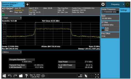
Plot 7-43. Occupied Bandwidth Plot (NR Band n30 - 10MHz 16-QAM - Full RB - Ant A)
