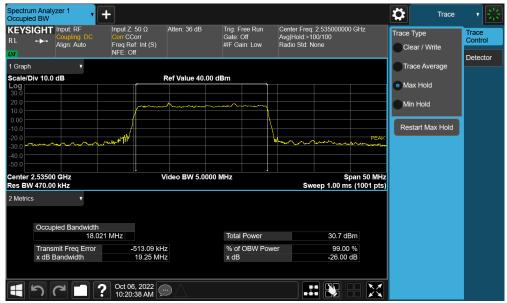
Plot 7-65. Occupied Bandwidth Plot (NR Band n7 - 20MHz π/2 BPSK - Full RB - Ant F)
