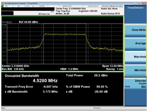
Plot 7-4. Occupied Bandwidth Plot (LTE Band 30 - 5MHz 16-QAM - Full RB - Ant A)
