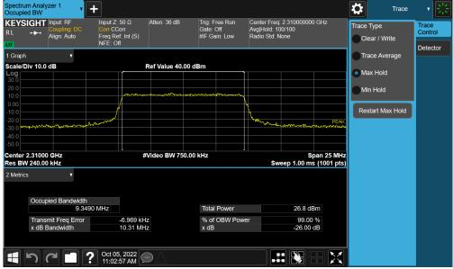
Plot 7-48. Occupied Bandwidth Plot (NR Band n30 - 10MHz QPSK - Full RB - Ant F)
