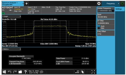
Plot 7-53. Occupied Bandwidth Plot (NR Band n7 - 20MHz π/2 BPSK - Full RB - Ant B)
