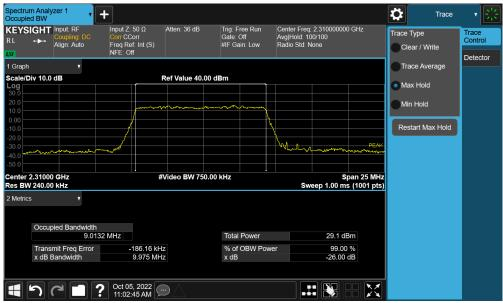
Plot 7-47. Occupied Bandwidth Plot (NR Band n30 - 10MHz π/2 BPSK - Full RB - Ant F)
